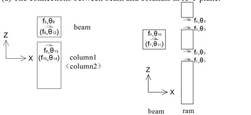
(b) The connections between beam and columns in X-Z plane.
