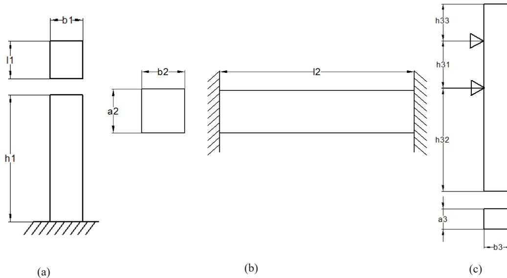
Fig.2 The equivalent models of the static stiffness in X direction.
