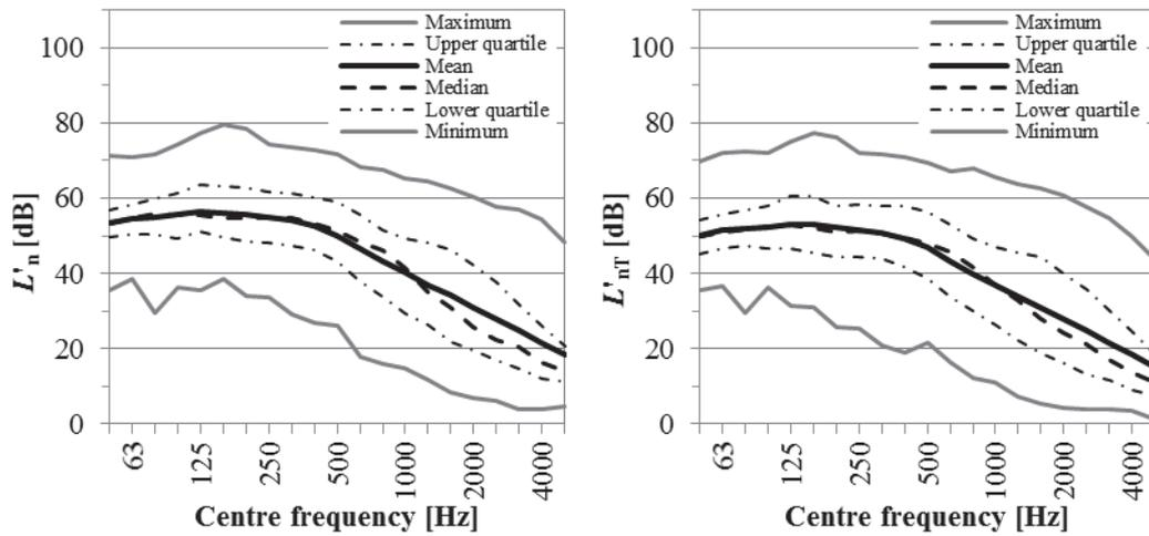
Figure 2 – Percentiles and mean values of the 110 measured normalized and standardized impact sound pressure levels  $L'_{n}$  and  $L'_{nT}$
