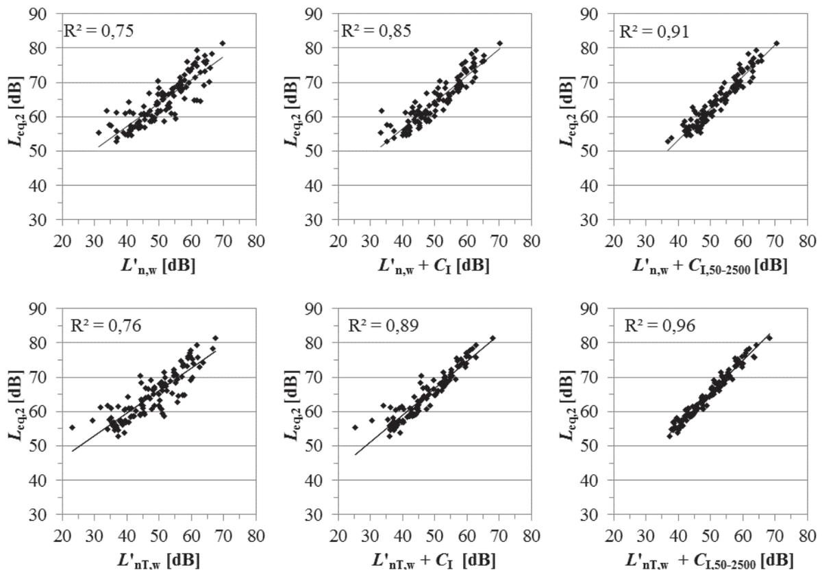
Figure 4 – Transmitted sound pressure levels  $L_{eq,2}$  as a function of the SNQs for impact sound insulation
