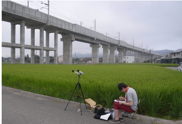
Figure 2 – The Hokuriku Shinkansen railway noise and vibration measurement
