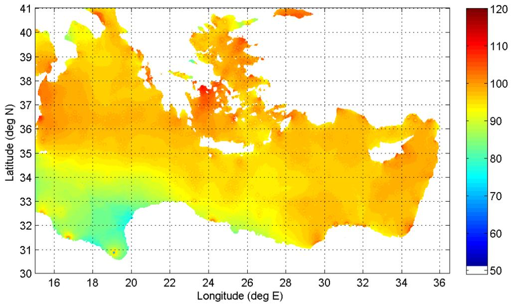
Figure 3. Predicted noise levels in dB re 1  $\mu$ Pa/Hz at a depth of 100 m.
