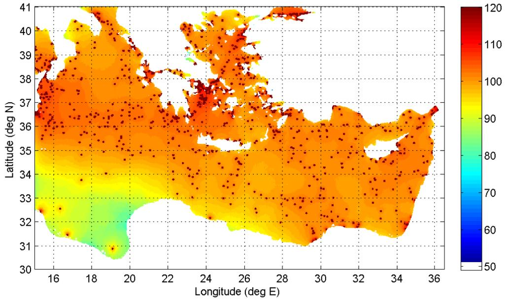
Figure 2. Predicted noise levels in dB re 1  $\mu$ Pa/Hz at a depth of 40 m.
