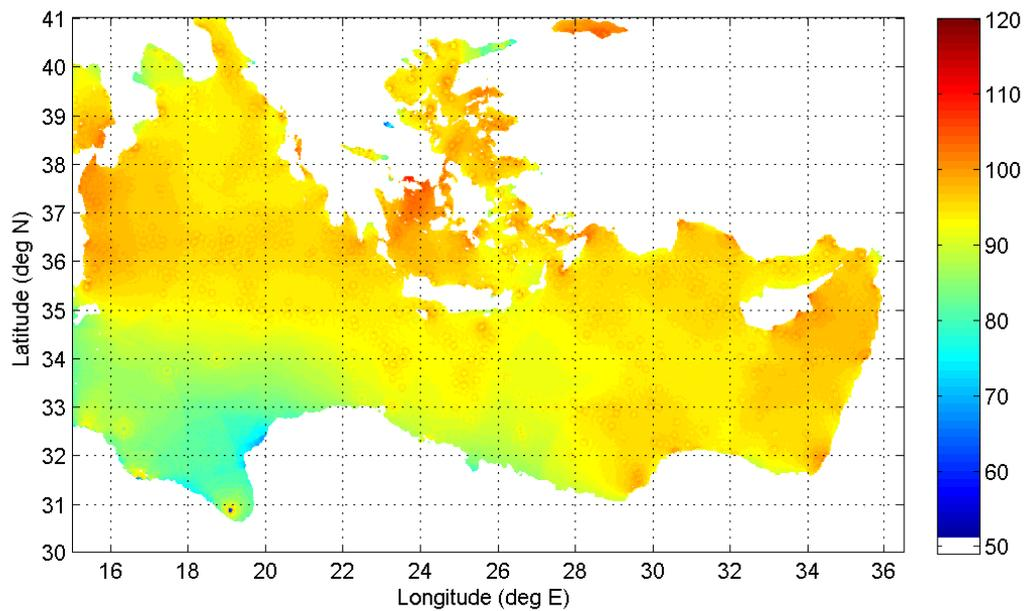
Figure 4. Predicted noise levels in dB re 1  $\mu$ Pa/Hz at a depth of 200 m.
