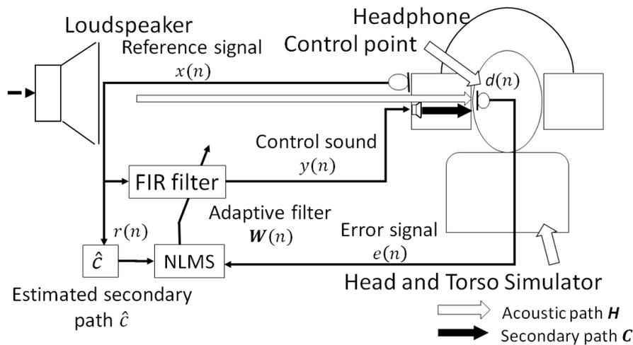
Figure 1 – Schematic of the system of a conventional active noise canceller.
