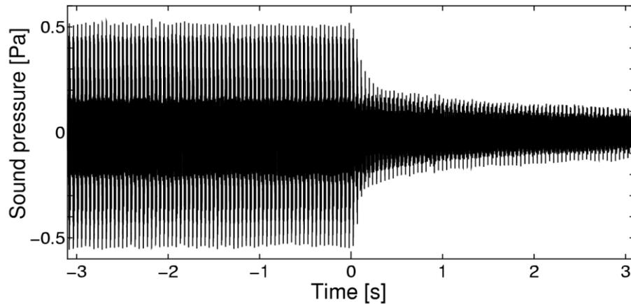
Figure 5 – Waveform of sound pressure received by the subject using the proposed active noise canceller in the case of T1W imaging noise.
