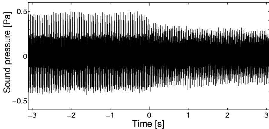
Figure 3 – Waveform of sound pressure received by the subject using the conventional active noise canceller in the case of T1W imaging noise.
