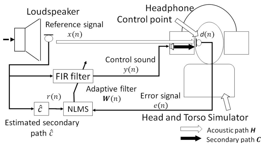
Figure 2 – Schematic of the system with the reference microphone for active MRI noise cancellation in the proposed position.
