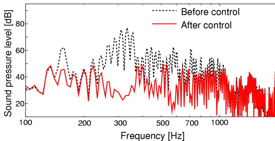
Figure 6 – Spectra of the noise received by the subject using the proposed active noise canceller in the case of T1W imaging noise.
