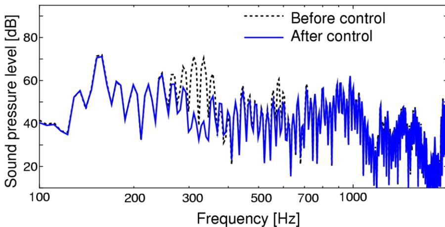
Figure 4 – Spectra of the noise received by the subject using the conventional active noise canceller in the case of T1W imaging noise.
