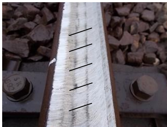
Figure 4 – Rail surface roughness by the present method
