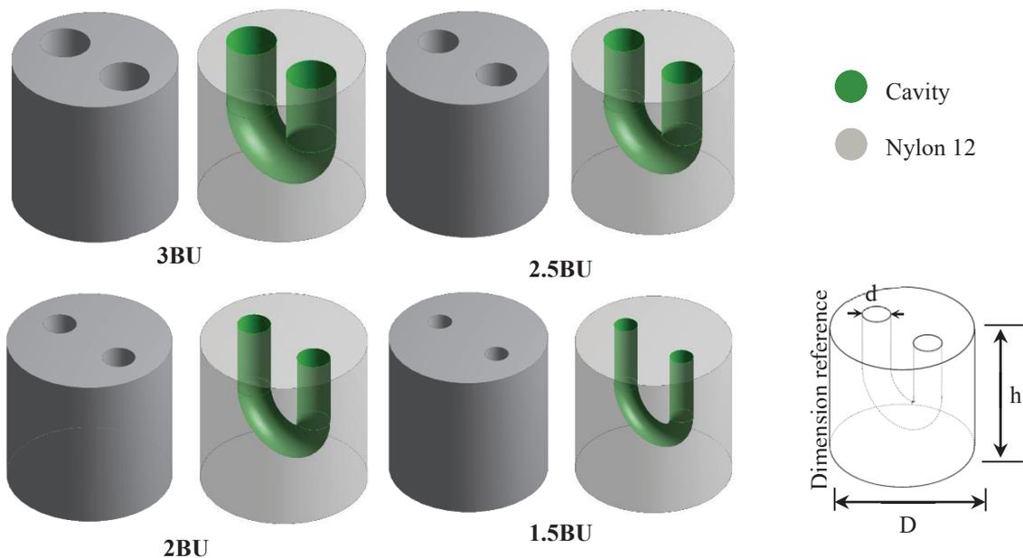
Figure 2 - Designs of the test specimen considered
