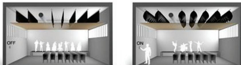
Figure 3 – A number of absorber-rows are mounted in the ceiling around fire sprinklers, ventilation ducts etc.
