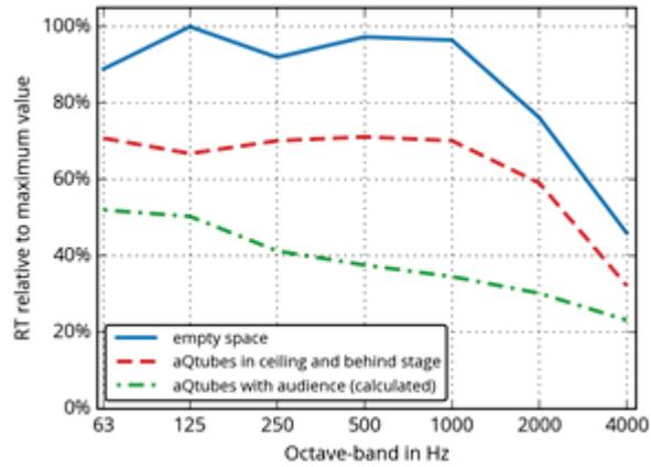
Figure 12 – Upper line indicates RT in empty space. In % due to discretion. Middle and lower line: tubes included. *One Direction* concerts, Amsterdam Arena 2014
