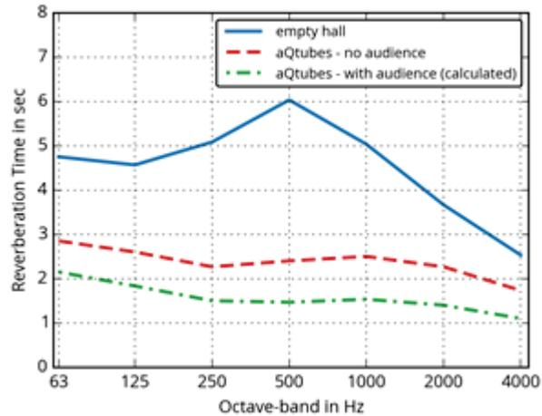
Figure 15 – Upper line indicates RT in empty space. Middle line: tubes included in hall. Lower line: calculated RT w. tubes and audience. Neue Nationalgalerie, Berlin 2015
