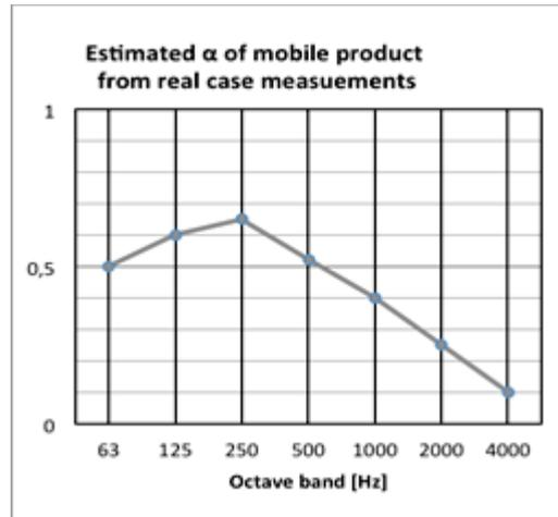
Figure 6 – Absorption coefficient, alpha, of mobile technology mounted as close as possible. Estimated from real case measurements; absorption effect only.
