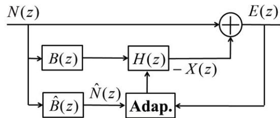
Figure 3 – Configuration reversed by regarding feedback path and noise control filter as linear system
