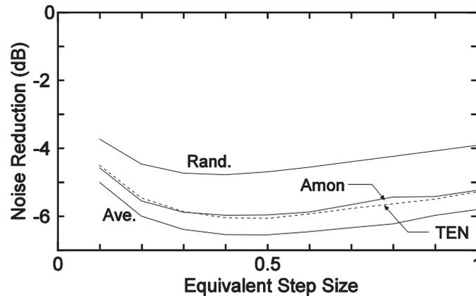
Figure 11 – Noise reduction effect provided by updating the estimation twice
