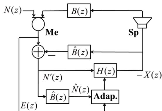
Figure 1 – configuration of feedback type active noise control system
