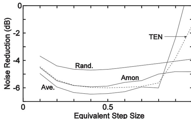
Figure 10 – Noise reduction effect curve provided by Sub-RLS algorithm
