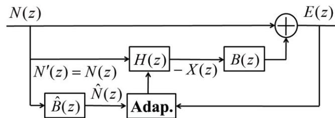
Figure 2 – Configuration simplified on the assumption that the feedback path is completely cancelled
