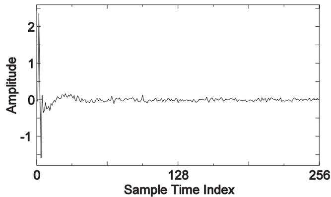
Figure 5 – Impulse response of feedback path measured by using TD307 (FUJITSU TEN)
