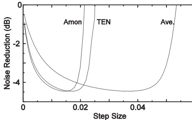
Figure 9 – Noise reduction effect curves calculated by applying NLMS algorithm to impulse response calculated using exponential decade regular random number
