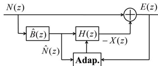
Figure 4 – Fundamental configuration of feedback type active noise control system shown in Fig.1
