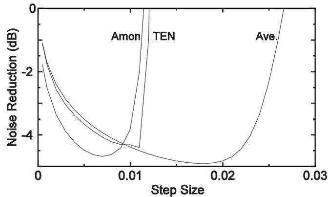
Figure 7 – Noise reduction effect curves calculated by applying NLMS algorithm
