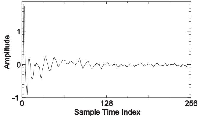
Figure 4 – Impulse response of feedback path measured by using ASW-2729D (Amon Ind.)
