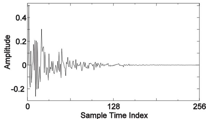
Figure 8 – Impulse response composed by using exponential decay regular random number
