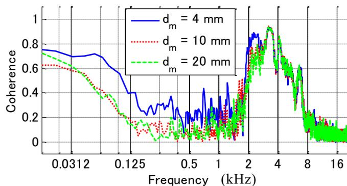
Figure 15 – Amplitude of complex coherence  $|\gamma_c(\omega)|$
