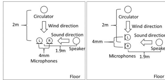
Figure 14 – Configuration of the equipments
