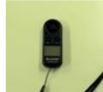
Figure 5 – Wind speed meter
