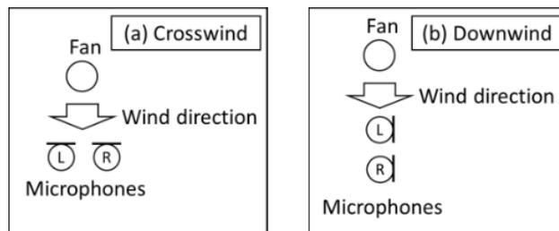
Figure 6 – Definition of the wind direction
