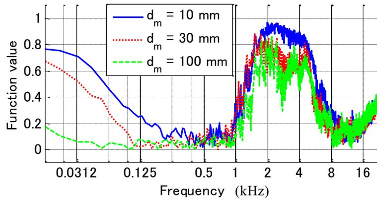
Figure 8 – Complex coherences for the microphone spacing (Downwind,  $v_w = 2.2$  m/s)
