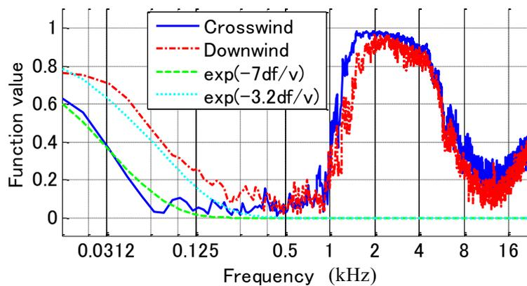
Figure 9 – Comp. coherence vs. wind direction ( $d_m = 10$  mm,  $v_w = 2.2$  m/s)
