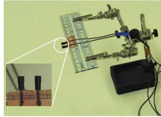
Figure 2 – Microphone array
