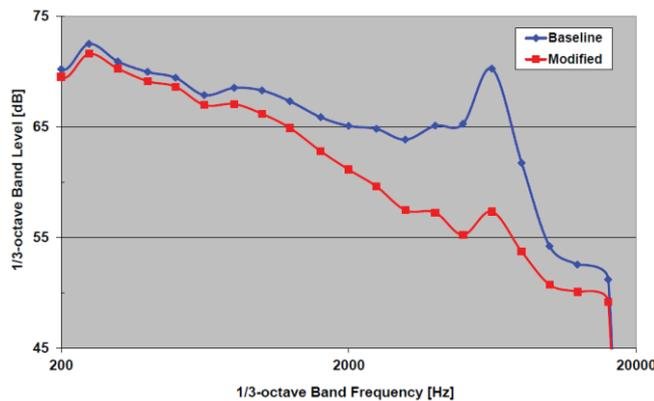
Figure 6 – Noise reduction potential by means of low noise side edge with flow velocity 50 m/s,  $\alpha = 5^\circ$ , 1/3-octave-band sound pressure spectrum with the microphone array measured.
