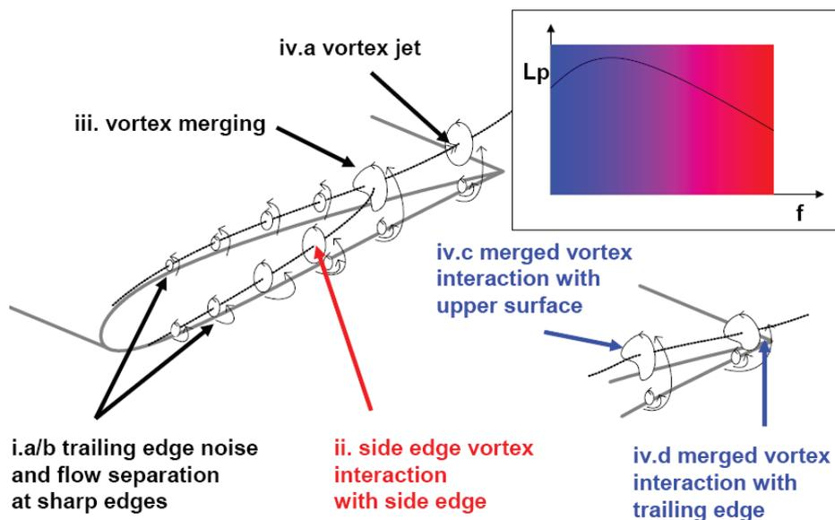
Figure 3 – Simplified scheme for the flap side edge local flow field.
