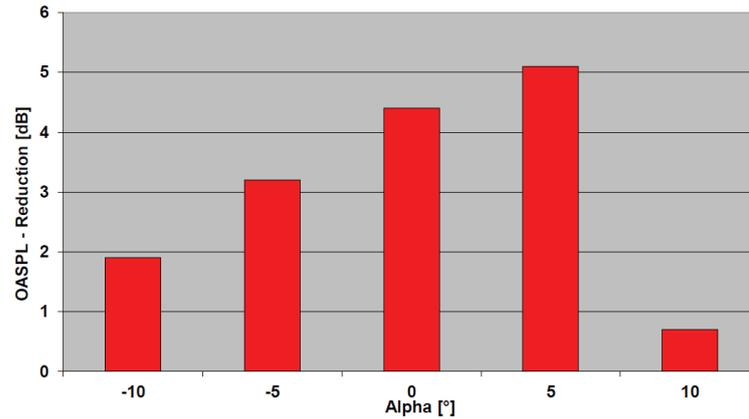
Figure 7 – Reduction of the total sound pressure level dependent on the angle of incidence alpha.
