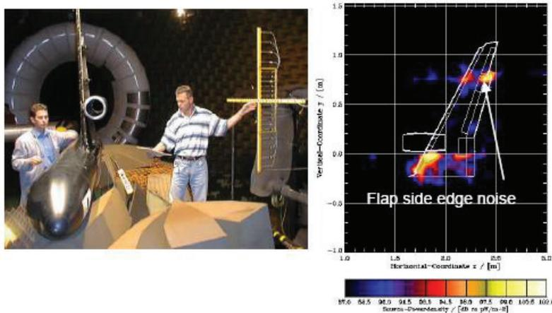
Figure 1 – Flap Side Edge Noise identified by microphone array technique in the wind tunnel
