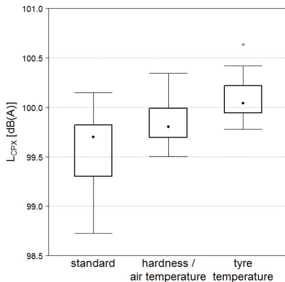
Figure 3 – distribution of corrected L<sub>CPX</sub> values, evaluated for the three different model methods
