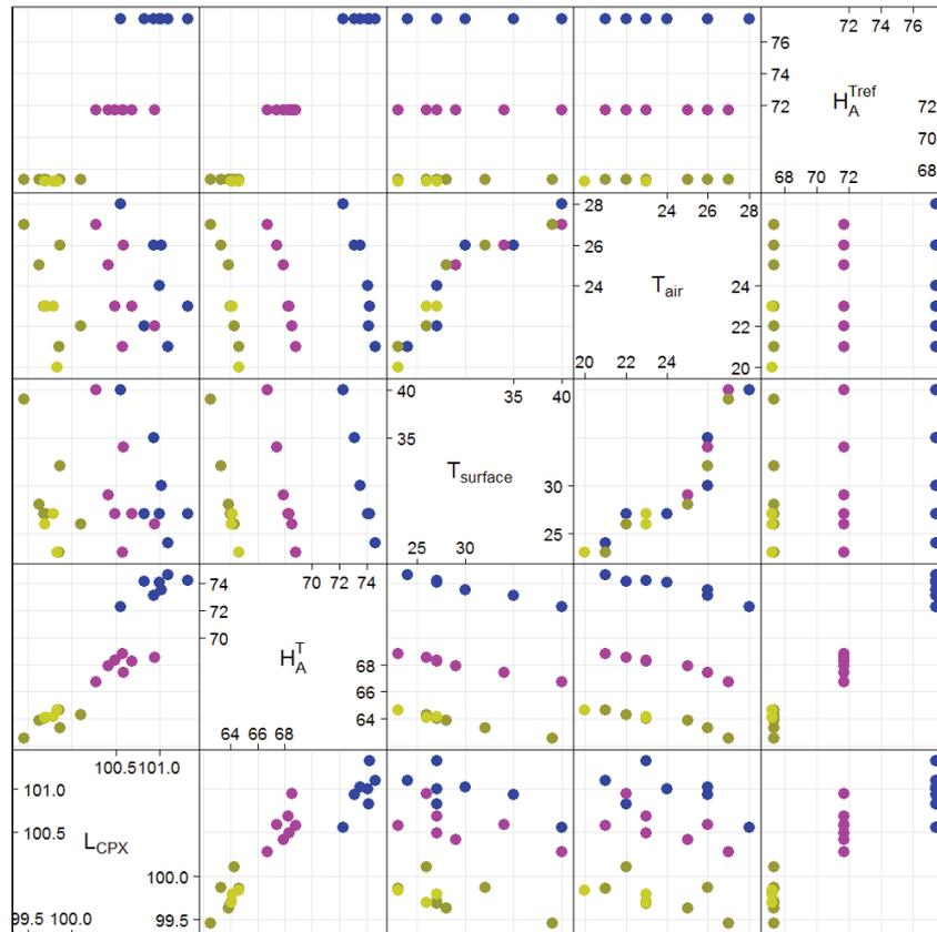
Figure 4 – scatter plot matrix of CPX sound pressure levels and relevant independent variables; the four measurement tyres are color-coded
