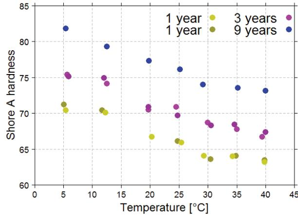
Figure 1 – temperature influence on shore A hardness of five different ASTM SRTT tyres; age of tyres is color-coded, their hardness increasing with increasing age
