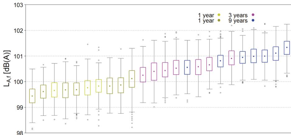
Figure 2 – distribution of uncorrected measured sound pressure values of the single measurement runs; the age of the tyres is color-coded in the figure
