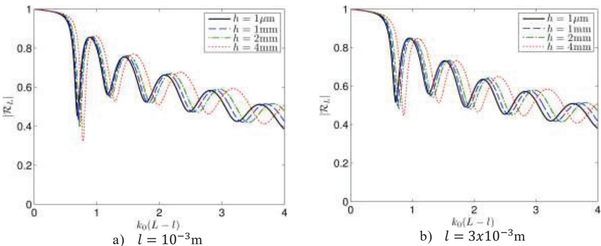
Figure 5 – Influence of the ring thickness on the retarding structure reflection coefficient for fixed number of rings/cavities and damping.
