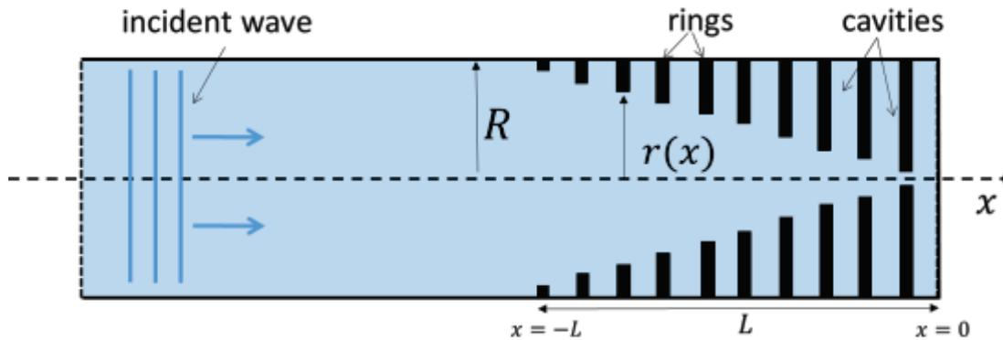
Figure 1 – Retarding structure to produce the ABH effect at the duct termination
