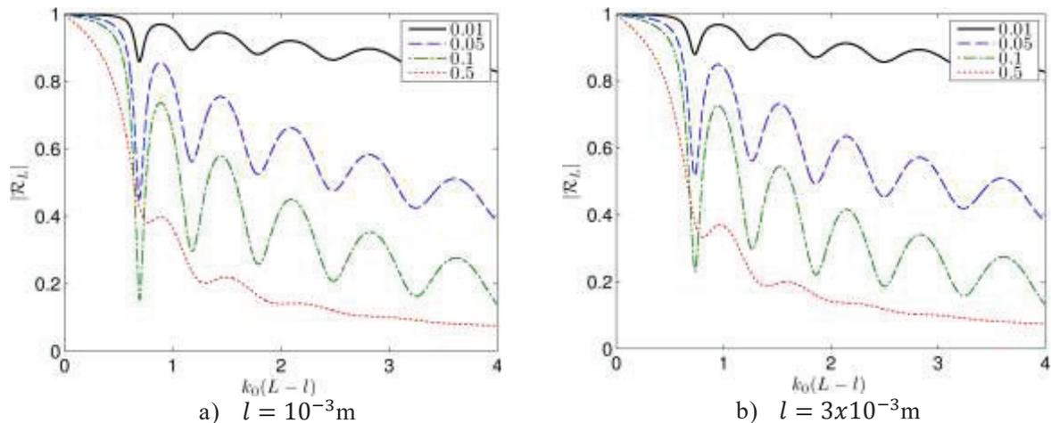
Figure 6 – Influence of damping on the retarding structure reflection coefficient for fixed number of rings/cavities and ring thickness.
