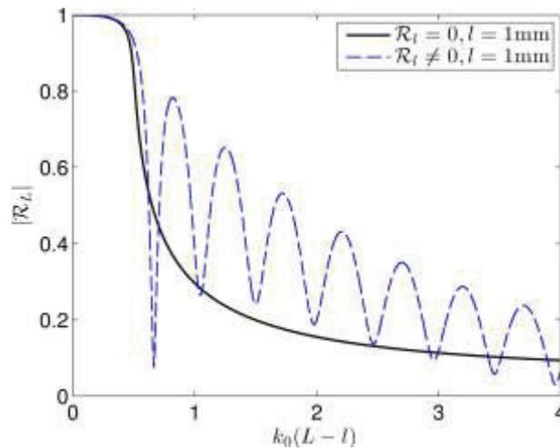
Figure 3 – Reflection coefficient  $R_L$  of the retarding structure for the cases of no reflection at the duct termination (black line) and rigid end termination (dashed blue line)
