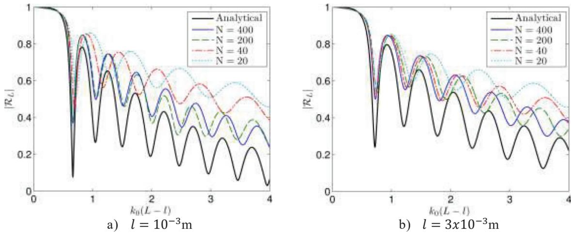
Figure 4 – Influence of the number of rings/cavities on the retarding structure reflection coefficient for fixed ring thickness and damping.
