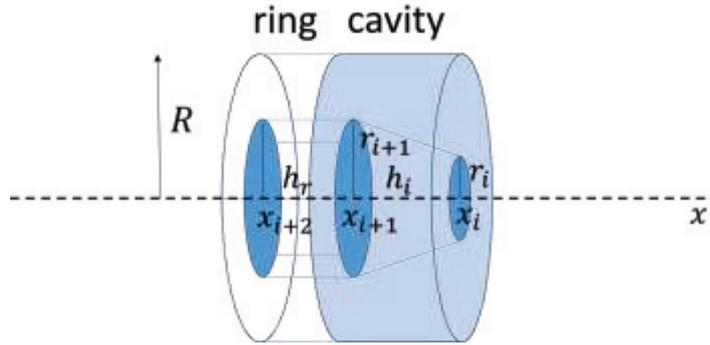
Figure 2 – Solid ring connected to a cavity limited by an inner virtual truncated cone surface and the duct walls.
