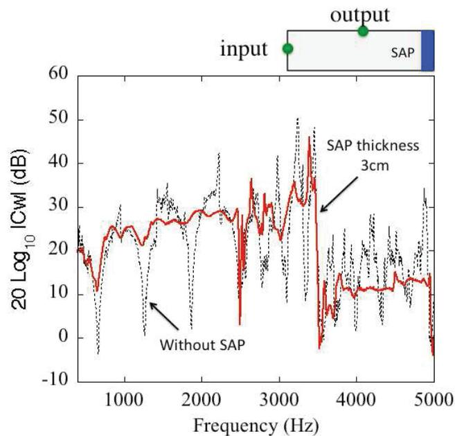
Figure 5 –When changing a SAP thickness
