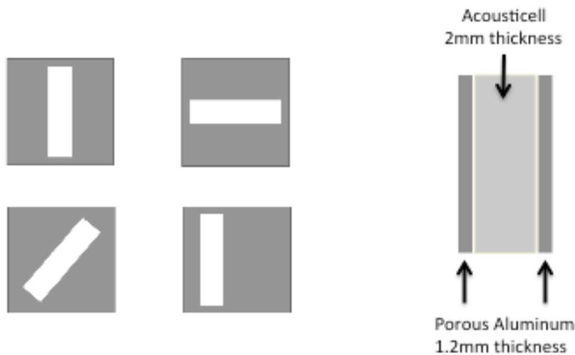
Figure 3 –The sound absorbing plate
