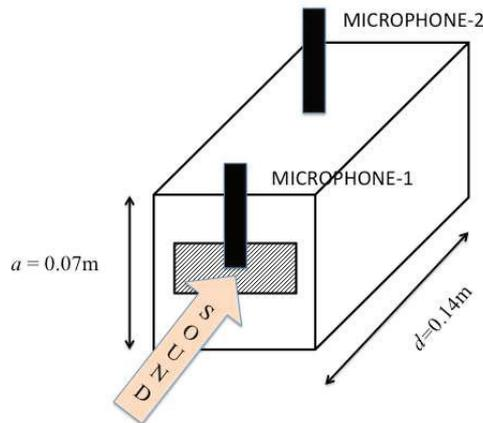
Figure 2 – Measurement apparatus
