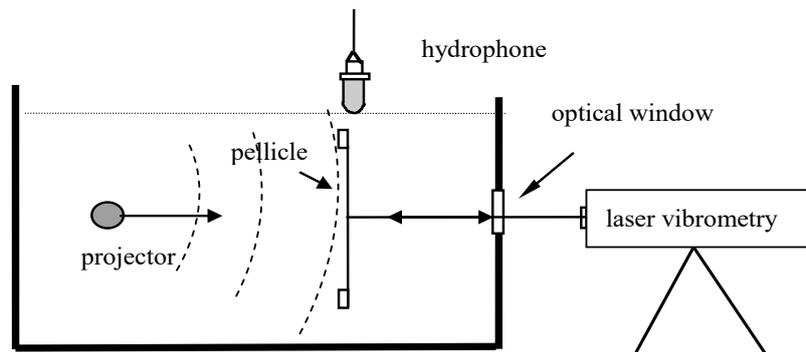
Figure 1 – Schematic diagram of calibration principle using optical method
