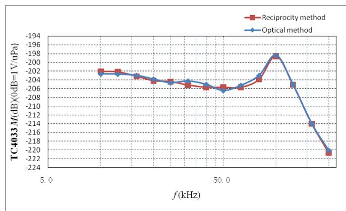
Figure 4 –Results comparison between the optical and reciprocal methods for TC4033
