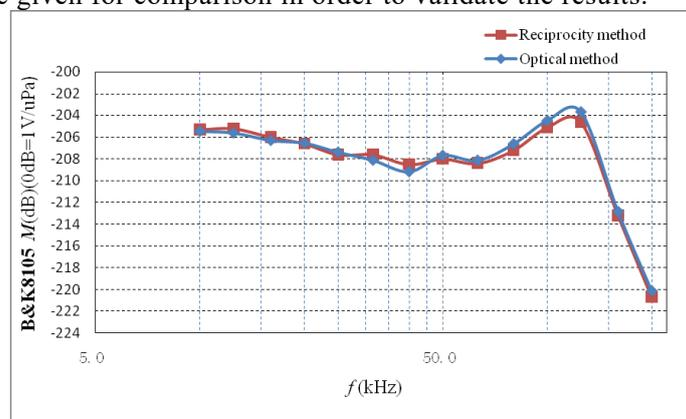
Figure 3 –Results comparison between the optical and reciprocal methods for B&K 8105
