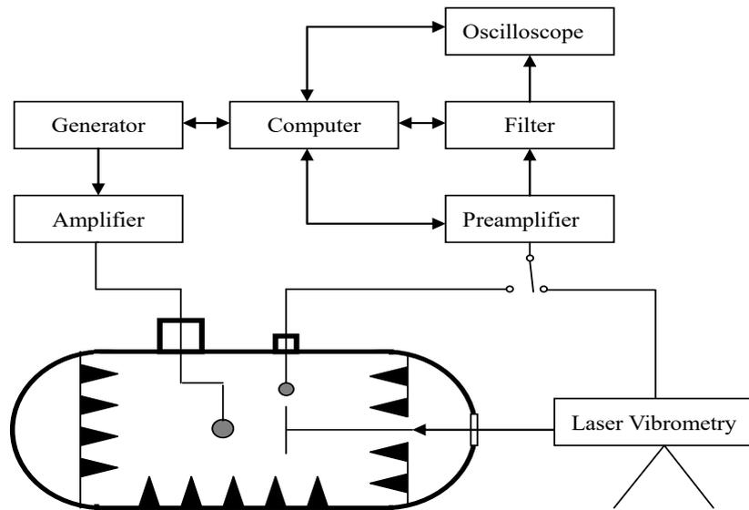
Figure 2 – Schematic diagram of the experiment facility
