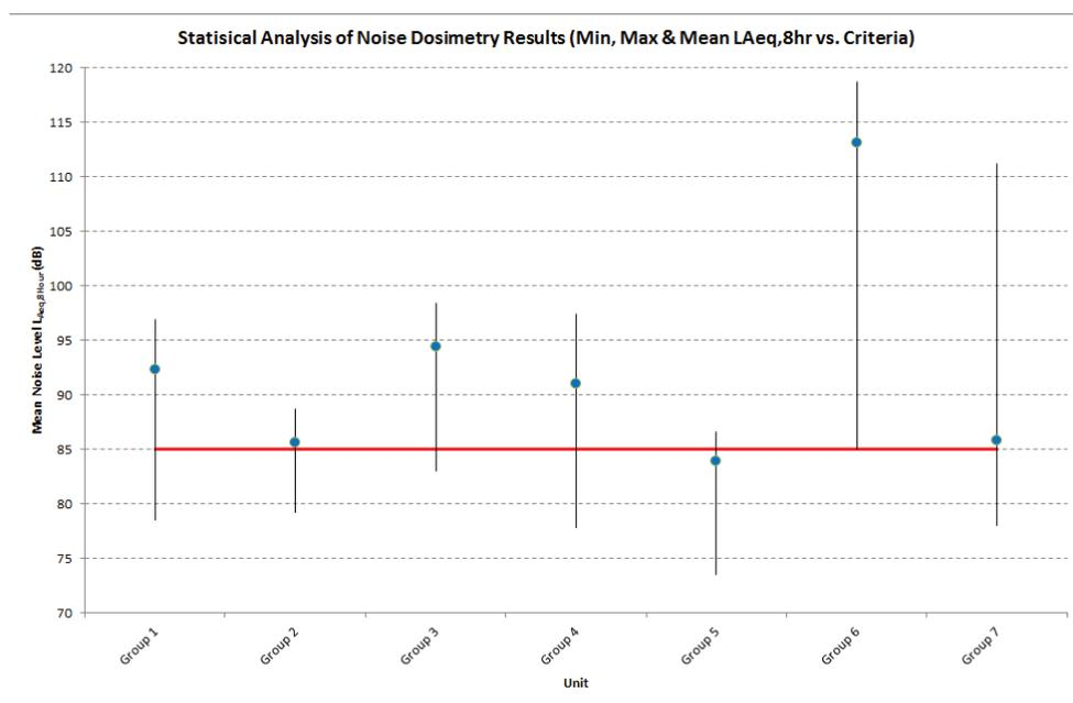
Figure 1 – Noise dosimetry statistical analysis for different sections at an ADF facility
