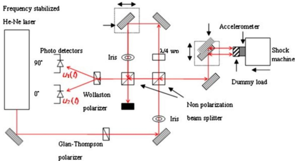
Figure-3 Illustration of optical interferometer
