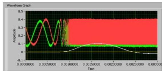
Figure-4 Interfering signal  $u_1(t)$  and  $u_2(t)$  of phase difference  $90^\circ$ .
