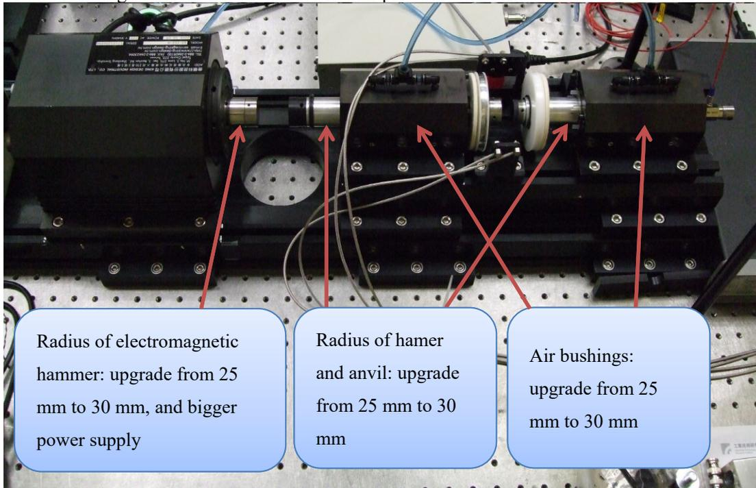
Figure 2 –Upgrade the shock level activating module
