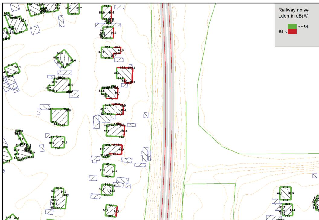
Figure 1. Results from a noise calculation of railway noise. Houses with façade noise levels greater than 64 dB (Lden) are eligible for noise insulation.
