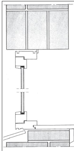
Figure 4. Cross section of a window with two-layer glass (1)
