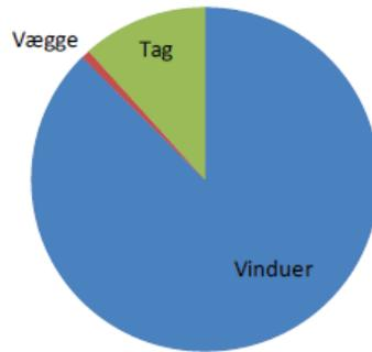
Figure 3. Distribution of the transmitted sound energy on windows, roof and walls (1).
