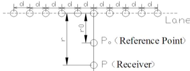
Figure 3 - Line sound source discretization
