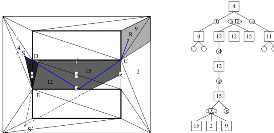
Figure 2 - An example of beam tracing
