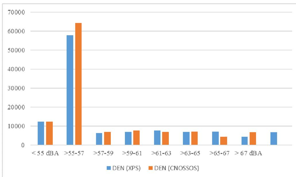
Figure 7 – Comparison of noise exposure of population figures (Lden) applying different noise calculation guideline to Trento agglomeration
