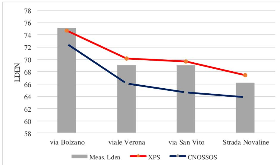
Figure 6 – Comparison of results given by XPS 31-133 and CNOSSOS\_EU Road for n.4 test locations
