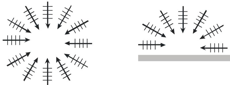
Figure 1 – 2D illustrations of full spherical isotropy (left) and hemispherical isotropy (right).
