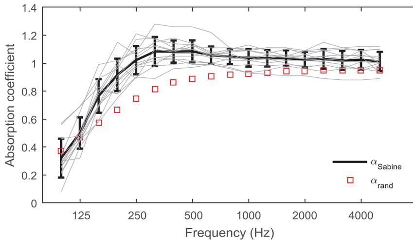
Figure 3 –  $\alpha_{Sab}$  of a 10 cm mineral wool with rigid backing measured in 13 chambers. The error bar: standard deviation and grey lines: individual chamber data.  $\alpha_{rand}$  based on Miki’s model and local reaction (28).
