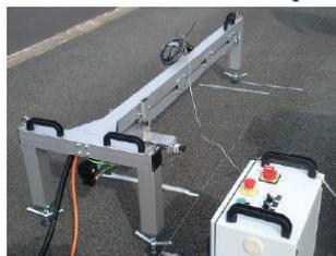
Figure 2 – 3D texture measurement system
