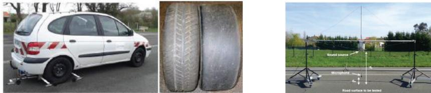
Figure 1 – Left: Test vehicle and tyres – Right: absorption measurement system
