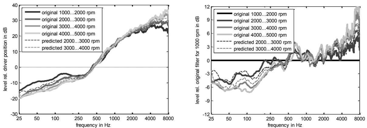
Figure 3 – Prediction of intermediate rpm states; left: filter frequency responses relative to driver position; right: filter frequency responses relative to filter response for 1000...2000 rpm.
