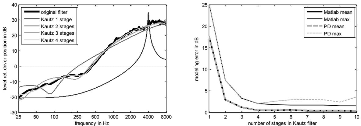
Figure 2 – Modeling of filter using Kautz filters (average 6-cyl. exterior back); left: frequency response of original filter and Kautz filters with different numbers of stages; right: mean/max modeling error for Matlab and PD real time implementation in dependence of number of Kautz stages.
