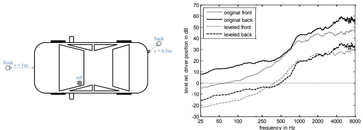
Figure 1 – Simultaneous recording of interior/exterior engine noise; left: recording positions; right: exemplary original and leveled magnitude spectra of exterior noise relative to driver position.
