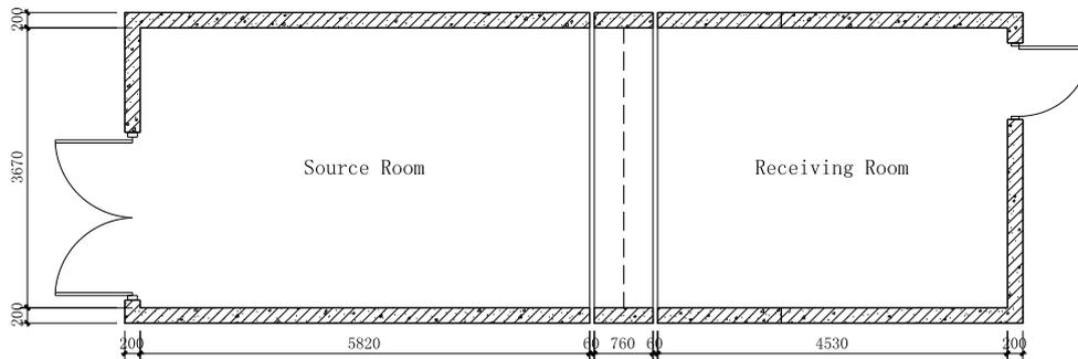
Figure 2 – Sound insulation test chambers
