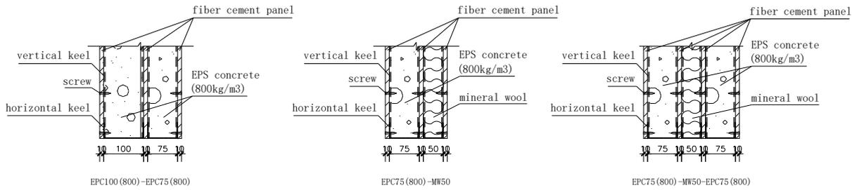
Figure 10 – Structure of multilayer walls
