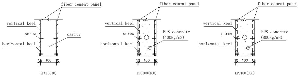
Figure 4 – Structure of walls with different concrete density
