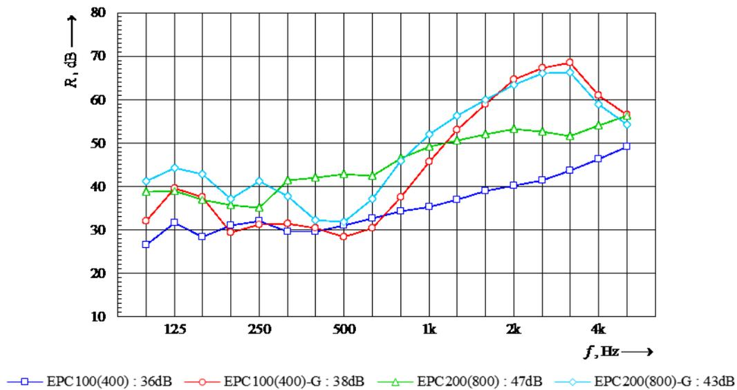
Figure 9 – Sound reduction index of walls with and without attached plasterboards
