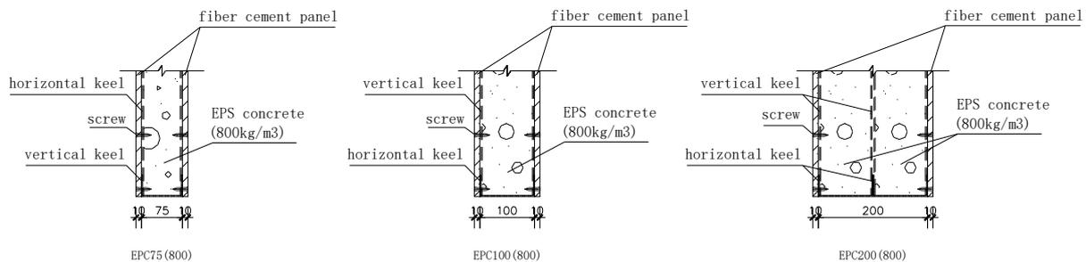
Figure 6 – Structure of walls with different concrete thickness
