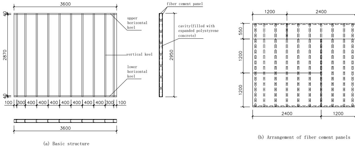
Figure 3 – Basic structure of the specimen
