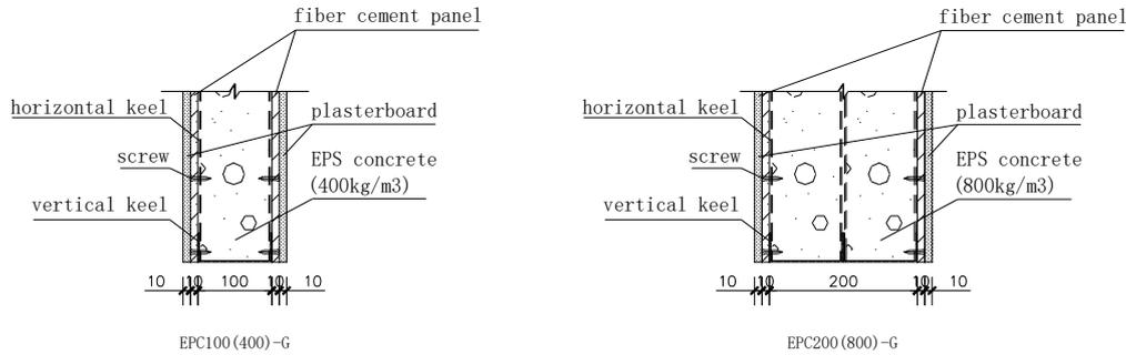
Figure 8 – Structure of walls with attached plasterboards
