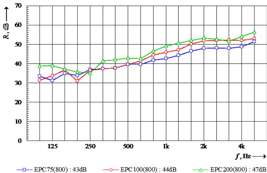
Figure 7 – Sound reduction index of walls with different concrete thickness
