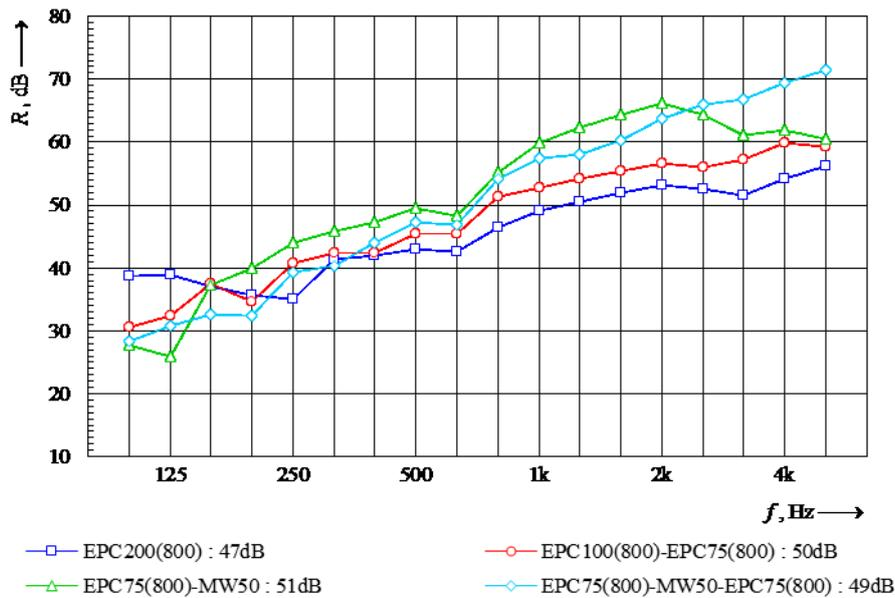
Figure 11 – Sound reduction index of multilayer walls
