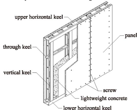
Figure 1 – Structure of lightweight steel gauge and lightweight concrete partition wall
