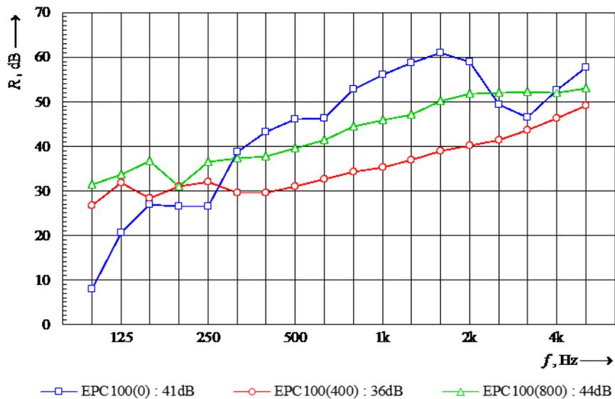
Figure 5 – Sound reduction index of walls with different concrete density
