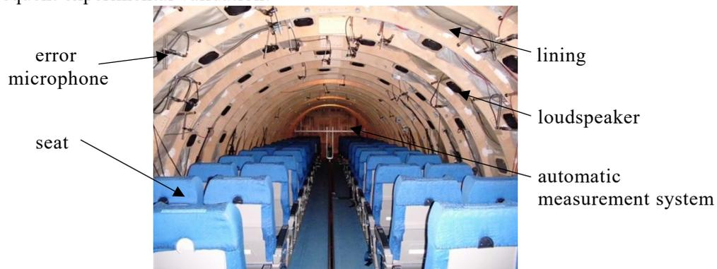
Figure 1 – Wooden fuselage mock-up © HSU/UniBwH
