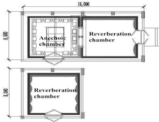
Figure 1 – Reverberation-anechoic chamber
