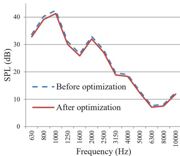
Figure 15 – SPL before and after sound package optimization
