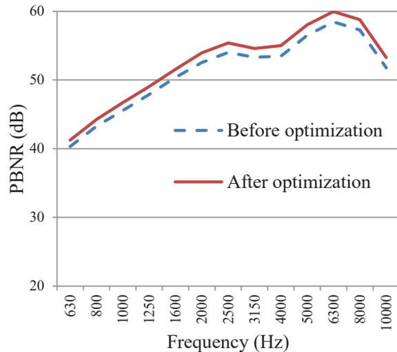
Figure 14 – PBNR before and after sound package optimization
