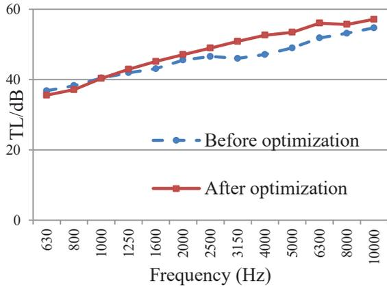
Figure 12 – The dash TL before and after sound package optimization
