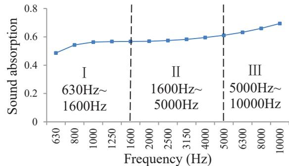
Figure 11 - Segments of sound absorption curve
