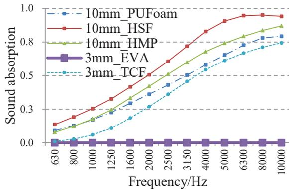
Figure 5 – Sound absorption of single material
