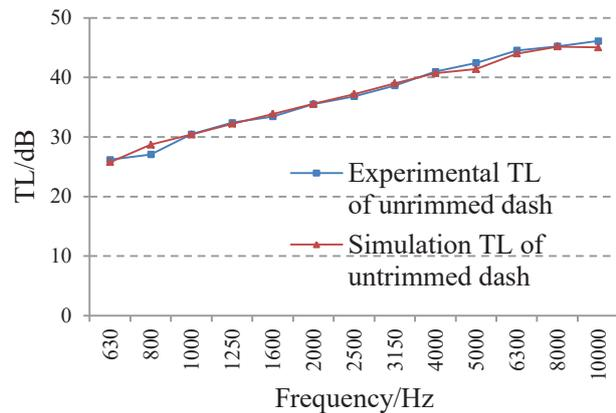
Figure 4 – Experimental TL and simulation TL of untrimmed dash
