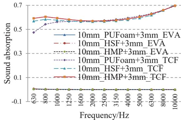
Figure 6 - Sound absorption of material combination
