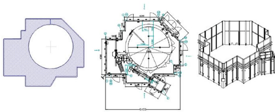
Figure 5: Model of a filling-machine (left) on basis of machine drawings (middle) and perspective views (right)
