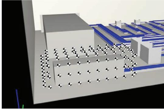
Figure 2 - Simulation of  $L_{WA}$ -determination with a box-type enveloping surface
