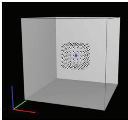
Figure 1 - Cubic arrangement of receivers - difference between  $L_{WA}$  of point source and  $L_{WA}$  determined is 0.9 dB
