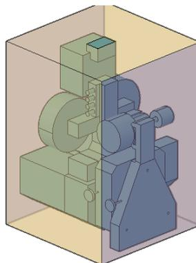
Figure 3 - The reference box enveloping the machine to be applied as machine-model
