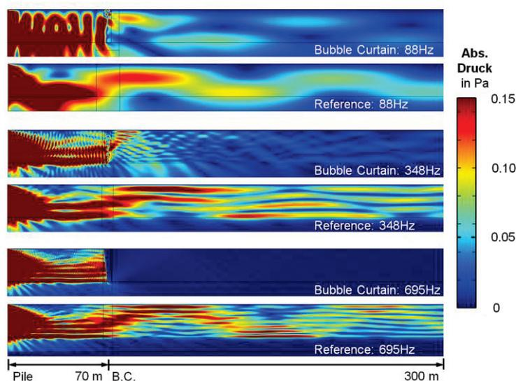
Figure 3 – Distribution of the absolute pressure for FINO3 with and without (i.e. reference) the bubble curtain for three frequencies
