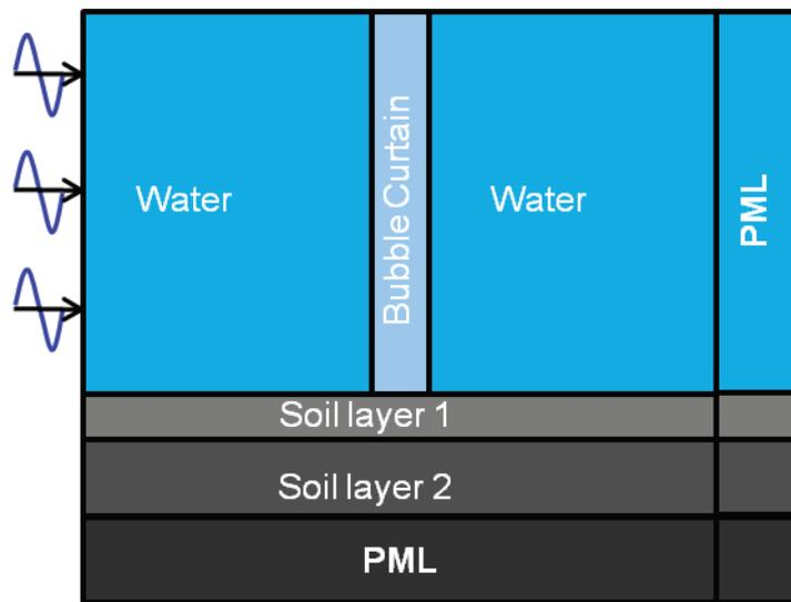
Figure 1 – Computational Domain with boundary conditions
