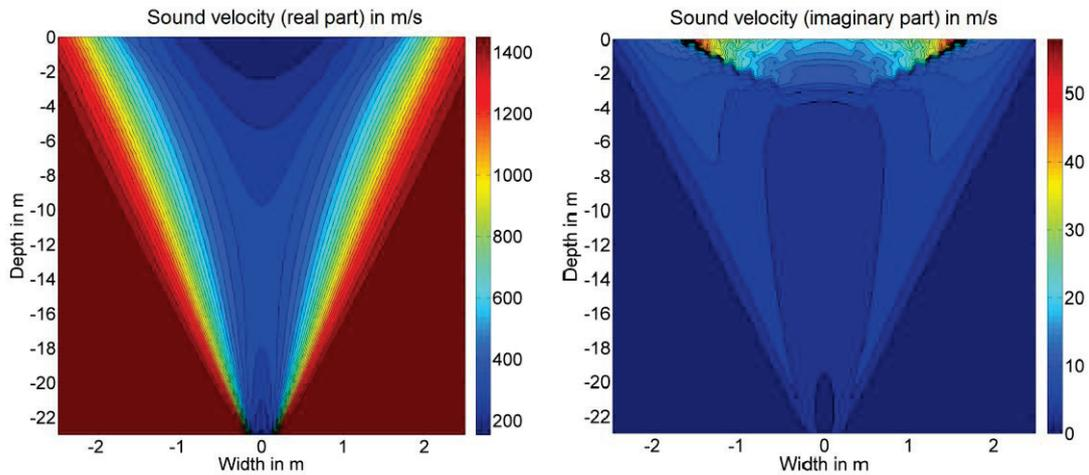
Figure 2 – Distribution of the sound velocity in the bubble curtain for a frequency of 348 Hz. (Left: real part, Right: imaginary part)
