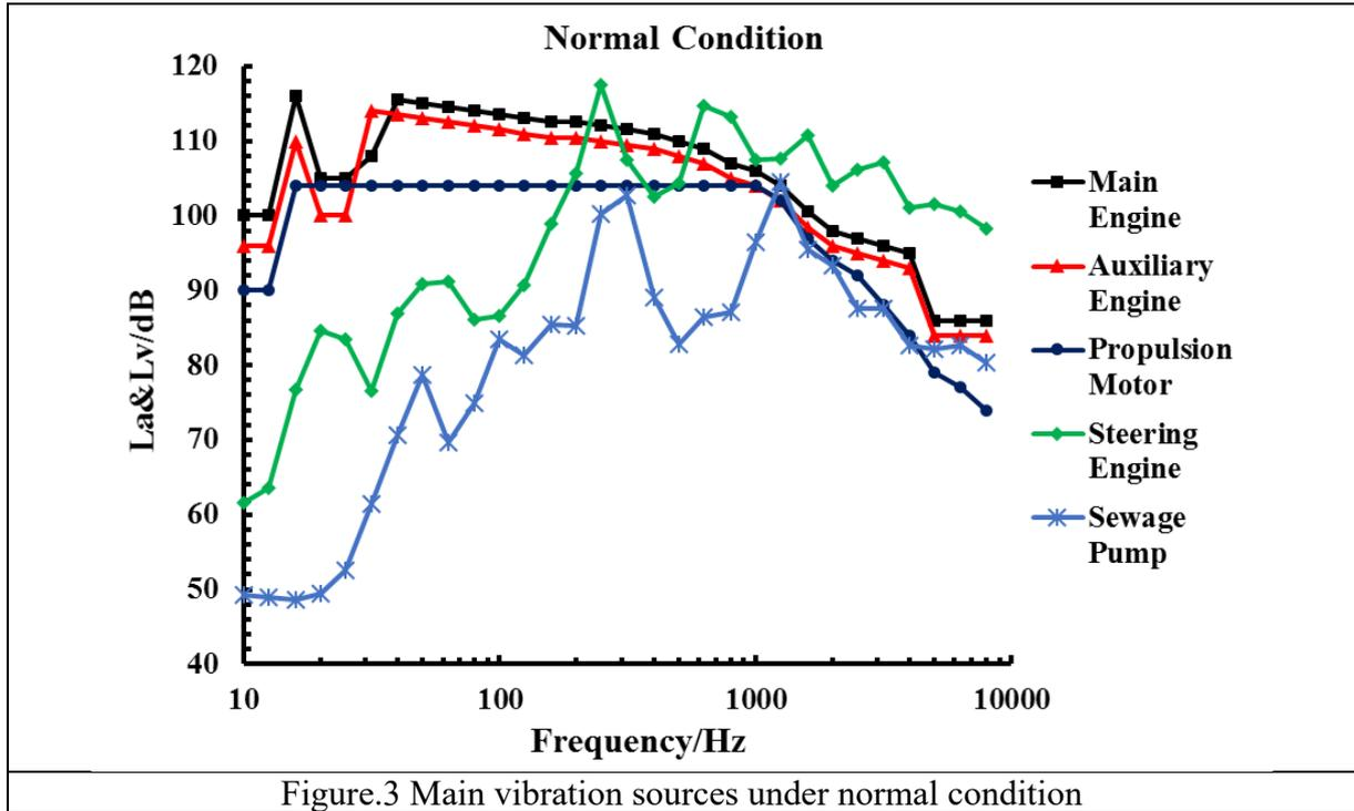
Figure.3 Main vibration sources under normal condition
