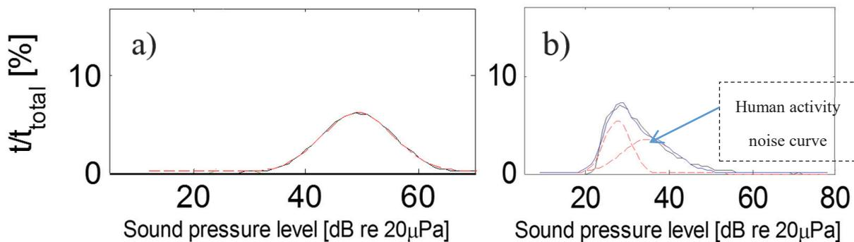
Figure 2 - Regression of a probability density function at 500 Hz, two different offices: a) a call center where one normal distribution gives the best fit and b) an engineer office where two normal distributions give the best fit. — : measured office noise, - - - : individual fitted normal distribution and — : overall fitted curve of office noise.
