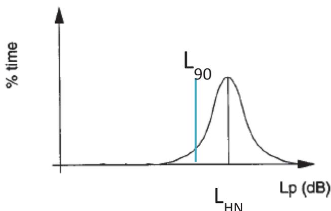
Figure 3 – Illustration of  $L_{90,HN}$  at the Gaussian distribution of human activity noise levels.
