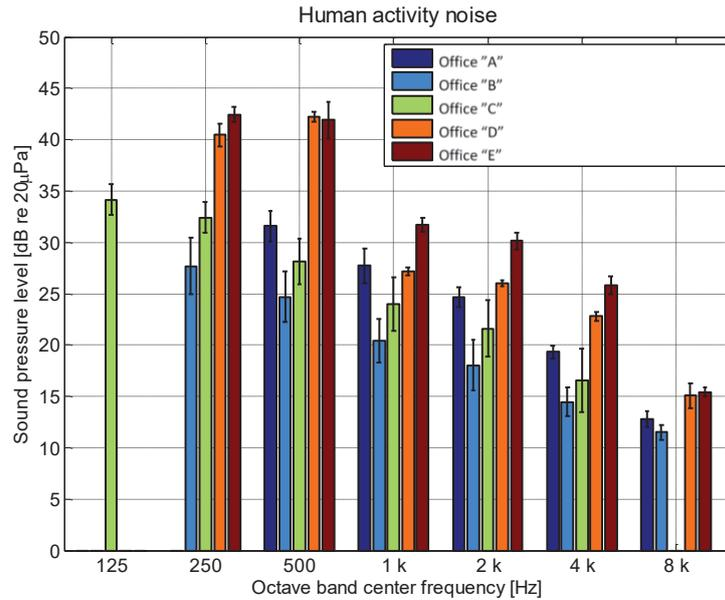
Figure 4 - Extracted human activity noise levels,  $L_{90,HN}$ , at seven octave bands in the five open plan offices.
