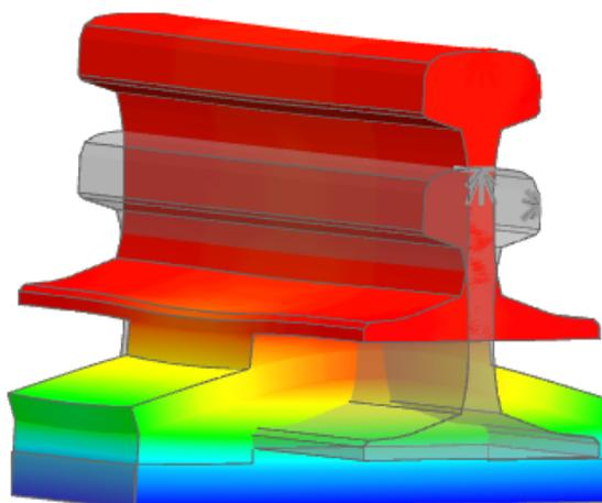
Figure 7 – Vertical mode at 220 Hz of a piece of rail (60 cm) on a double layer support
