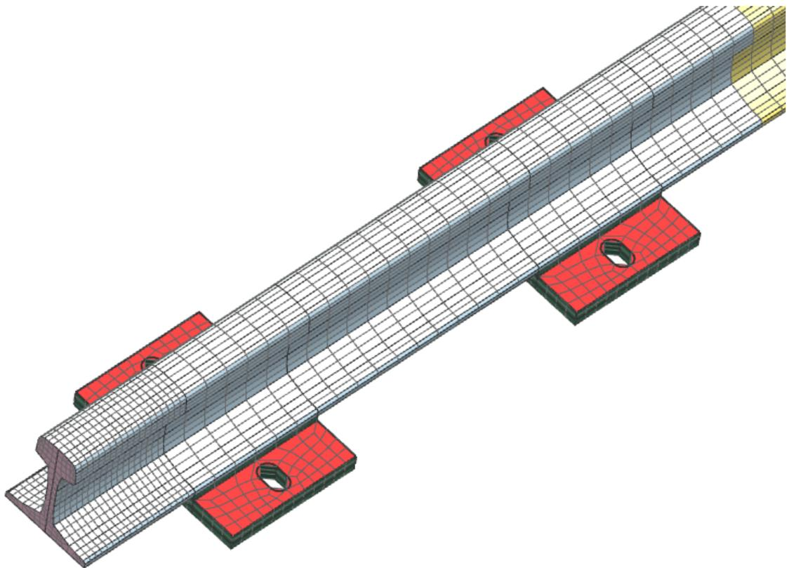
Figure 3 - FE-model of a rail with supports representative for slab tracks
