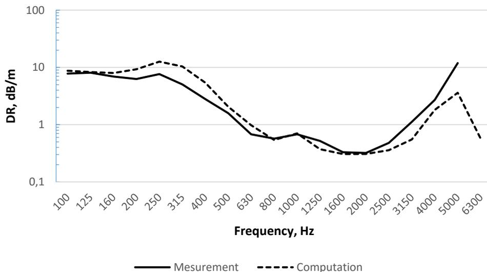
Figure 4 – Measured and computed vertical decay rates of a ballasted track
