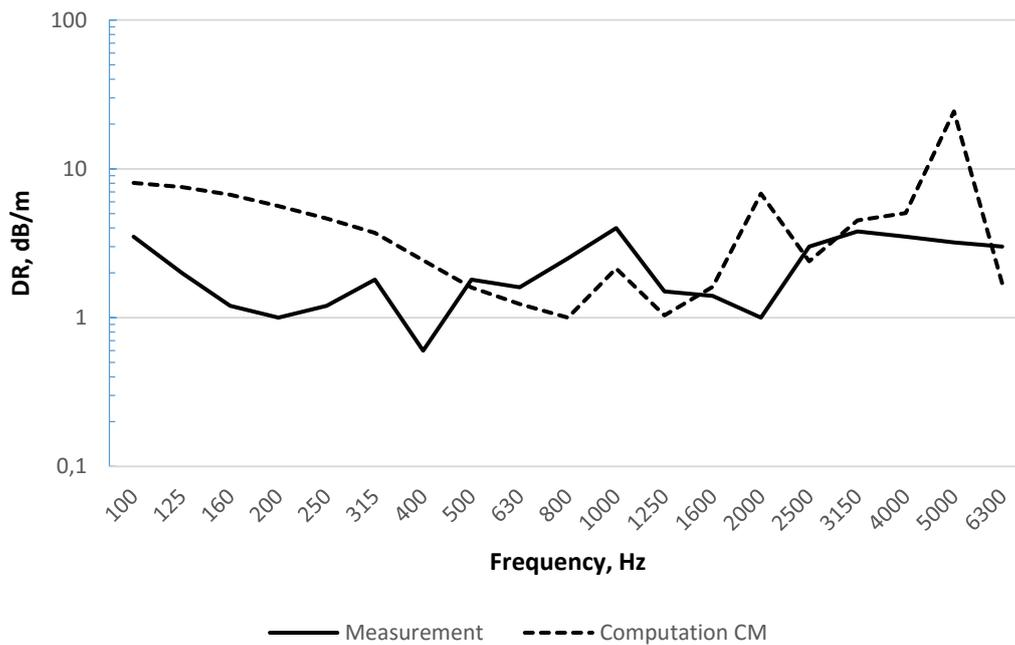
Figure 5 – Measured and computed vertical decay rates of slab track – simplified model
