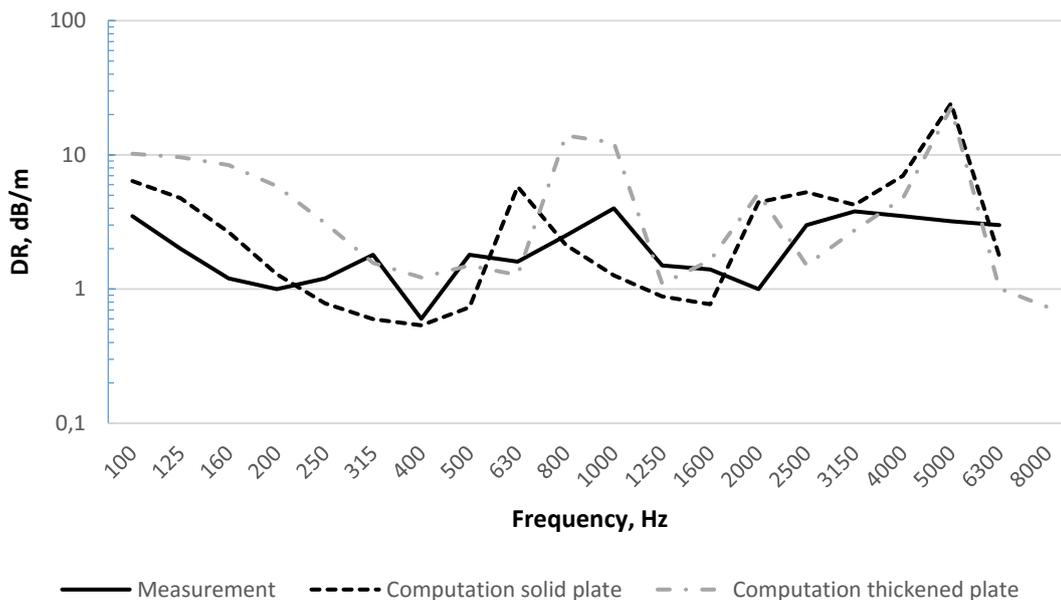
Figure 6 – Measured and computed vertical decay rates of a slab track – model including solid plates
