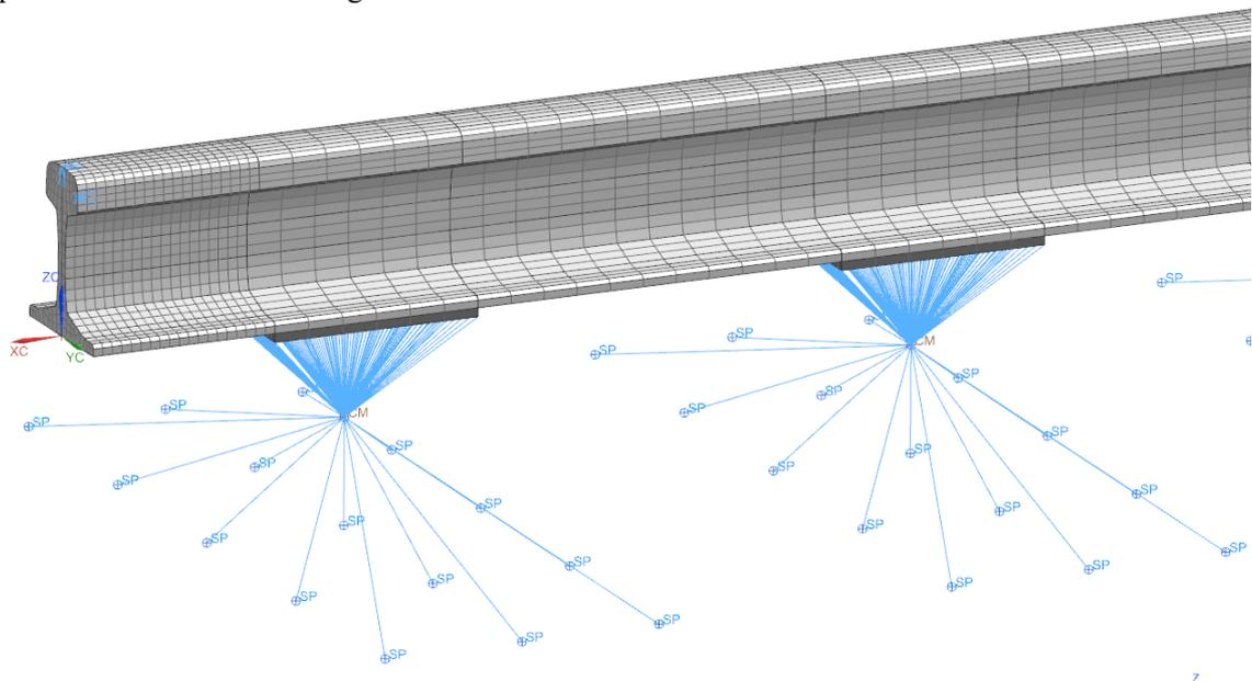
Figure 1 – FE model of a bi-bloc sleeper track.
