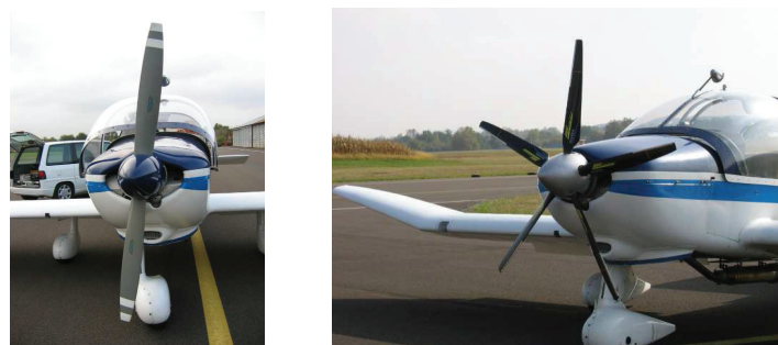
Figure 2 – Sensenich (left, reference) and ANIBAL (right) propellers mounted on a DR400 – 180R FGICU
