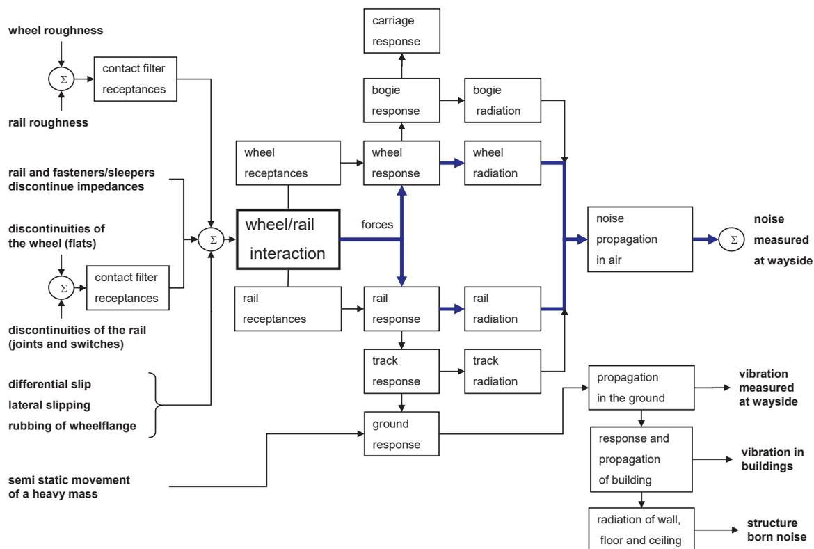
dGm<sup>R</sup> Diagram of the excitation mechanisms for noise and vibration.
