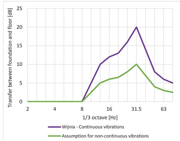
Figure 7 Measurement results of continuous vibration [5] and of non- vibrations
