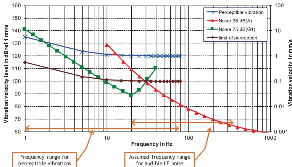
Figure 2. Graph with the sensitivity curves for humans on vibrations of floors of a dwelling and on low frequency structure-borne noise.
