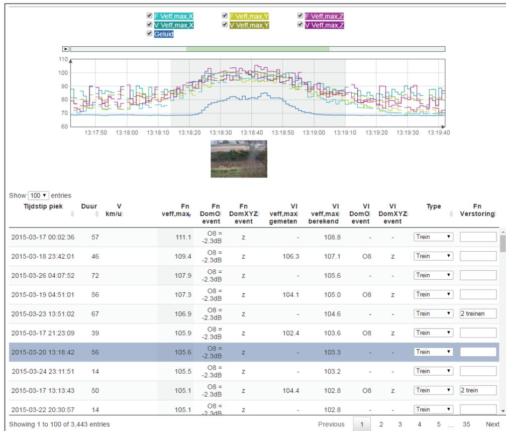
Figure 4 Example of the database of all the events. Data collected by Sensornet.
