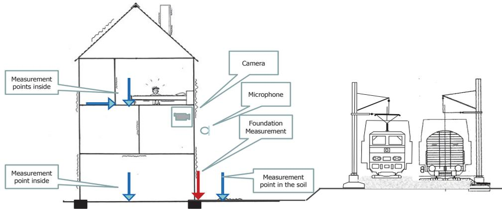
Figure 3 the measurement set-up in practice to determine the vibration of trains.
