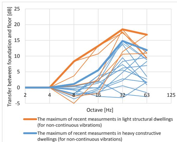
Figure 8 Measurement results according [3] divided into two groups, a group containing only dwellings with a massive building structure (blue) and a group consisting of only light structural dwellings (orange)
