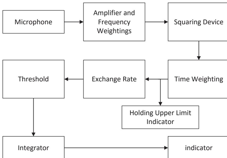
Figure 2 – Core Functional Blocks of a PSEM (ANSI 1.25)
