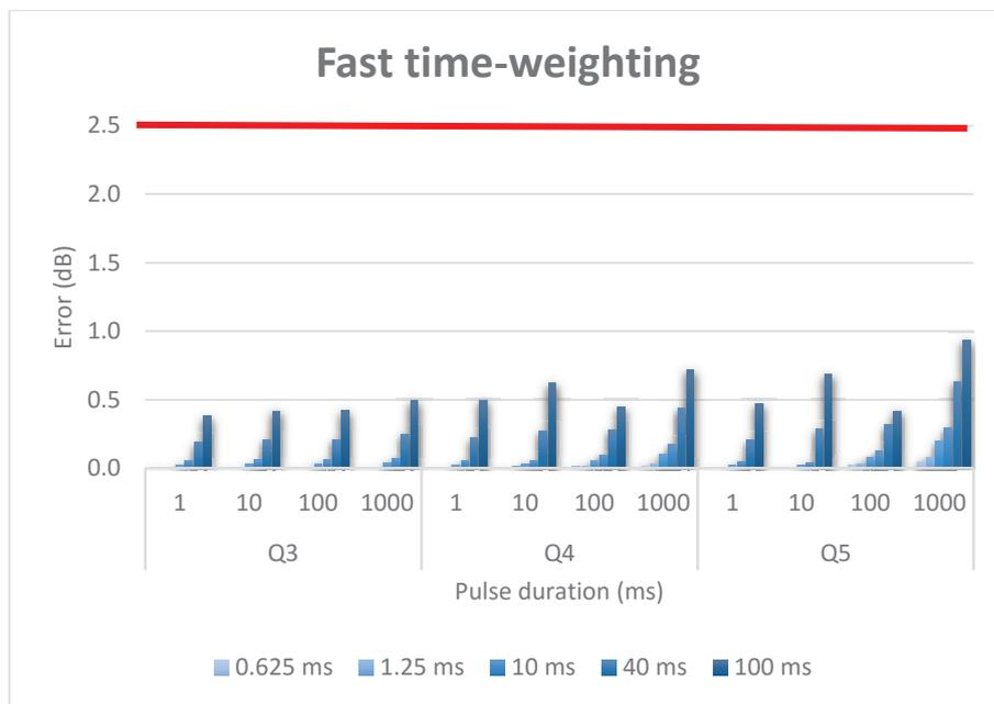
Figure 4a Error for tone burst response for Fast time weighted data.
