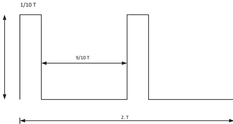
Figure 5 Injected Signal for the test described in ANSI S1.25 section 7.7 para. 3
