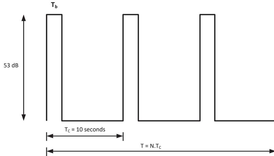
Figure 3 Injected Tone burst signal
