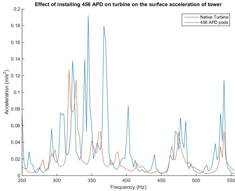
Figure 7 – Surface averaged normal acceleration of complete tower for the native turbine and for the turbine with 456 APD pods installed for frequencies between 250-550 Hz.
