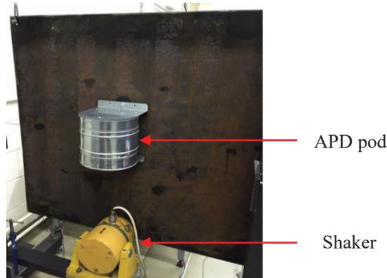
Figure 2 – Experimental set-up of the suspended plate with the APD pod placed in the center and the shaker. The acceleration was measured at 12 evenly distributed sensor locations on the other side of the plate.
