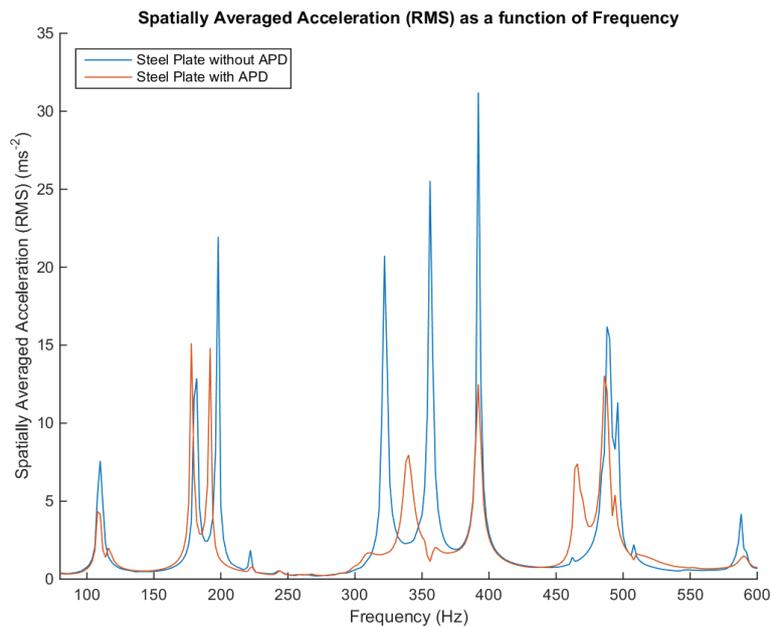
Figure 3 – Spatially averaged RMS acceleration as a function of frequency of the plate without and with the APD pod installed as shown in Figure 2. The installation of the APD pod reduces vibrations of the steel plate over a wide range of frequencies, from approximately 100 Hz to 600 Hz.
