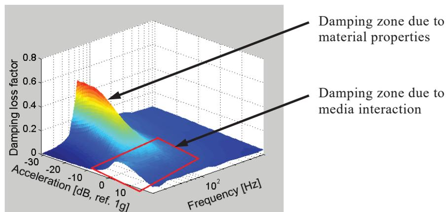
Figure 1 – Damping performance as a function of input frequency and acceleration level after (7)
