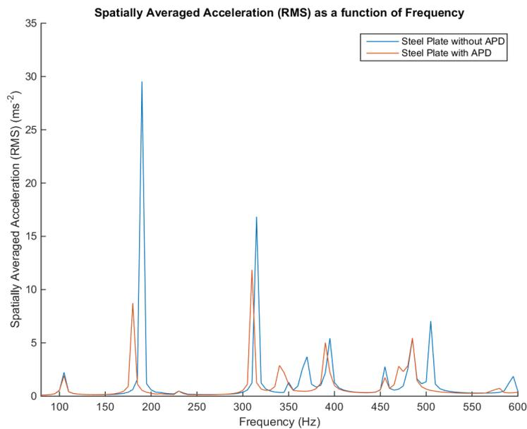
Figure 5 – Comparison of the spatially averaged RMS acceleration of the plate with the APD and the spatially averaged RMS acceleration of the plate without the APD pod for the modelled data.
