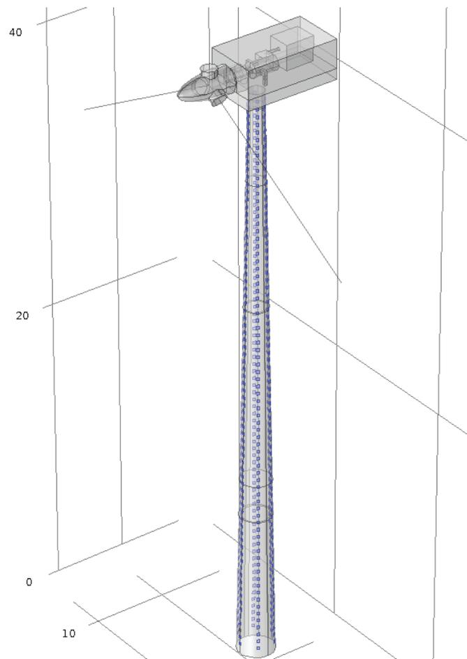
Figure 6 – Zoomed geometry of the wind turbine with APD pods installed. The APD pods are marked in blue.
