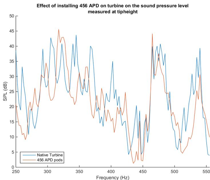
Figure 8 – Energy mean of the sound pressure level (SPL) in dB rel. 20 µPa modelled downwind, 30° off downwind, 60° off downwind and crosswind, at a distance equal to the tip height of the turbine for frequencies in the range 250-550 Hz.
