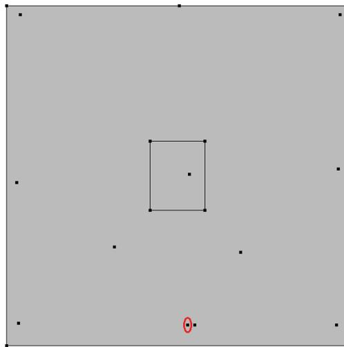
Figure 4 – Geometry of the simplified model, where the rectangle describes the APD pod placed on the metal sheet and the point with the red circle represents the shaker as a point source, as in the experiment described in section 3.1. All other points represent sensors as placed in the experiments.
