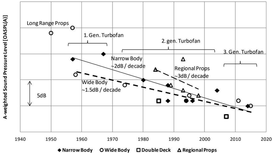
Figure 1: Evolution of cabin noise in passenger aircraft
