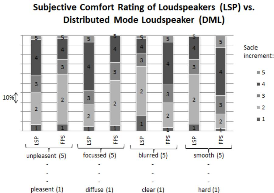
**Figure 8: Comparison of the sound quality of a distributed mode (DML) and a conventional cone loudspeaker integrated (LSP) in the passenger supply chain**
