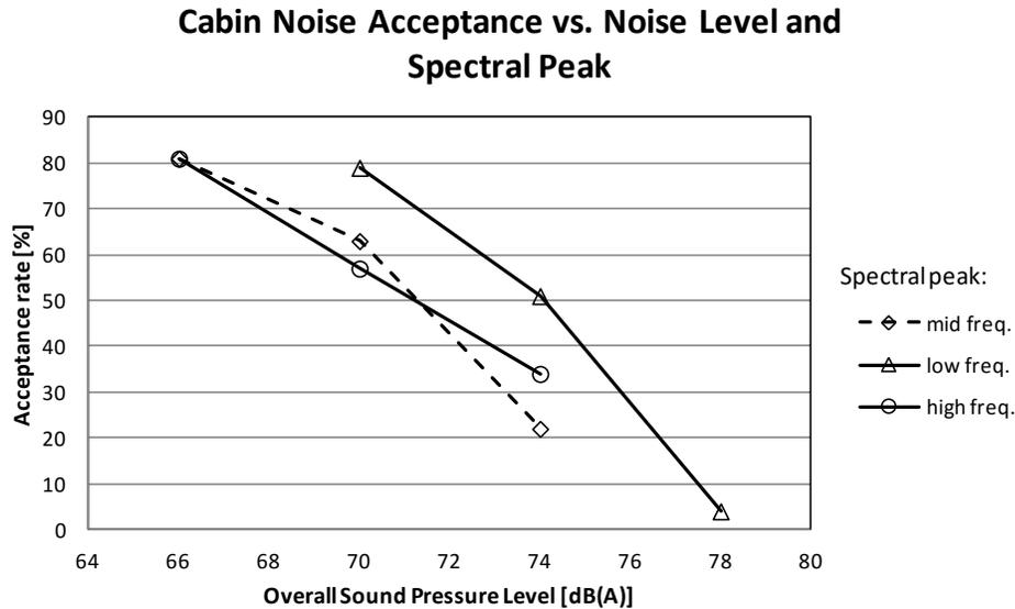
**Figure 5: Acceptance of cabin noise in relation to overall sound pressure level and frequency content**
