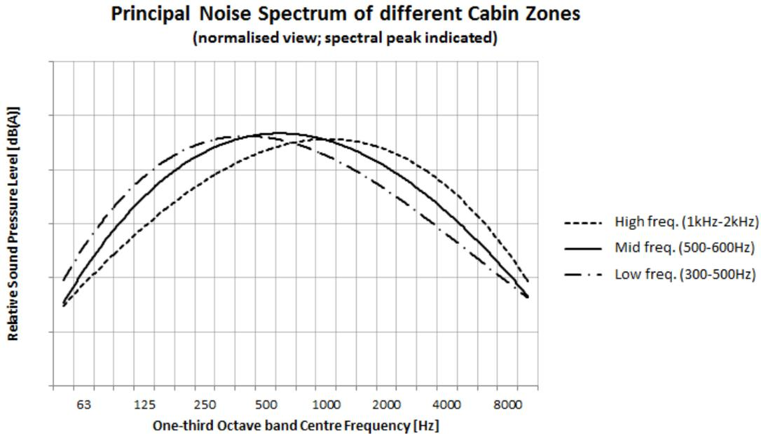
Figure 2: Principle noise spectra in different cabin zones a turbfan aircraft (wing mounted engines)
