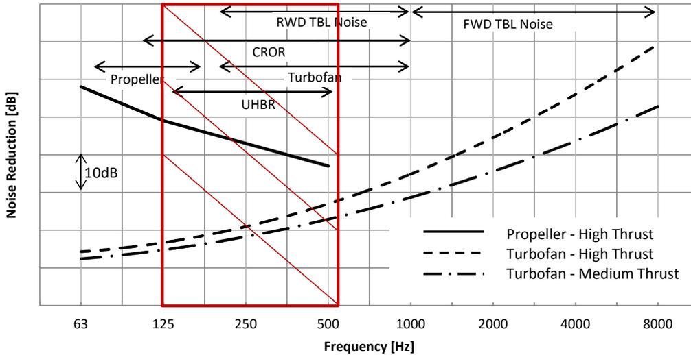
**Figure 8: State-of-the-art efficiency of noise reduction technologies**
