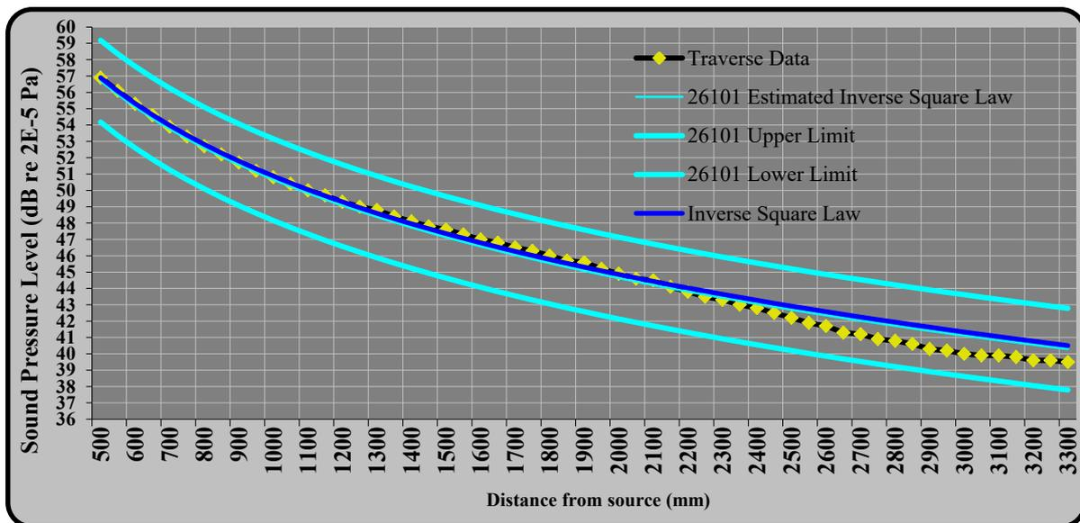
Figure 1: Large Hemi-Anechoic Chamber – ISO 26101 Curve Fit to 100 Hz
