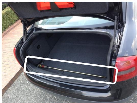
Figure 1 – Performance damper installed on a car
