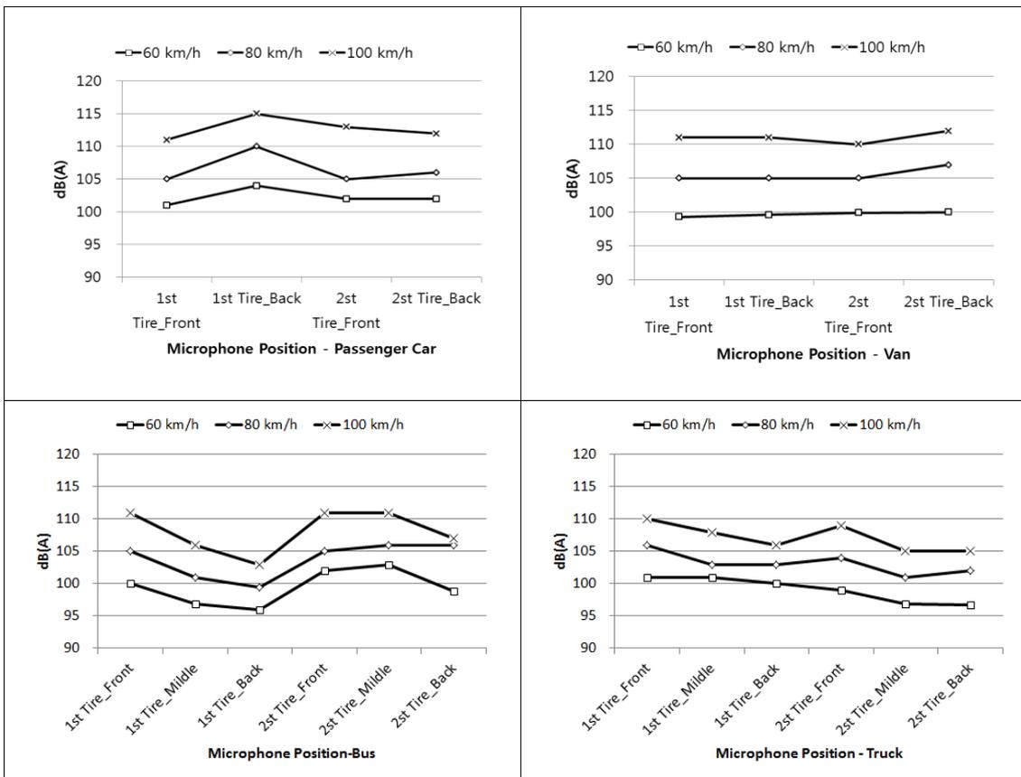
Figure 5 - Sound Pressure on Concrete Pavement by Microphone Position
