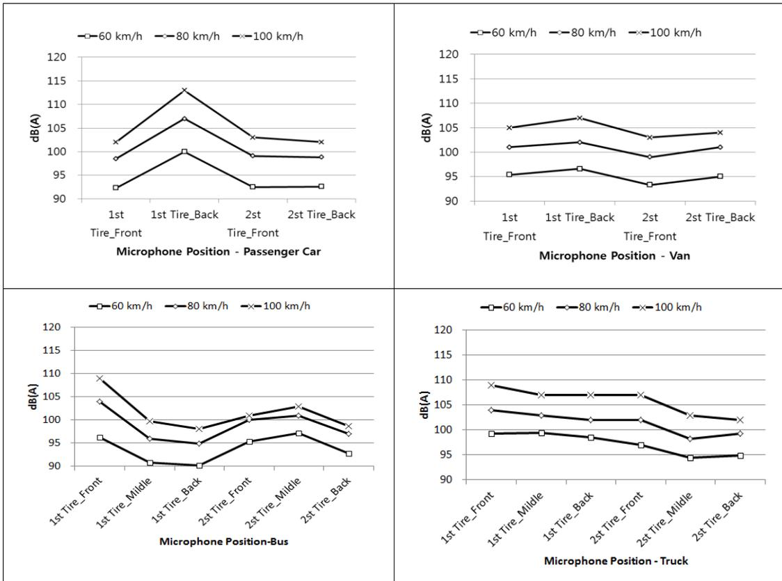
Figure 4 - Sound Pressure on Asphalt Pavement by Microphone Position
