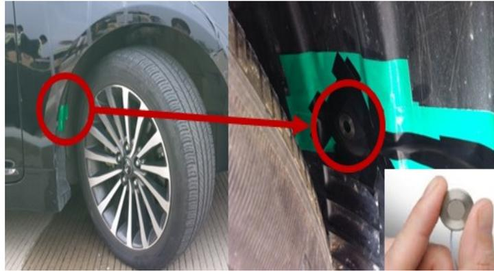
Figure 1 - Noise Measurement from Noise Source (NCPX Method)
