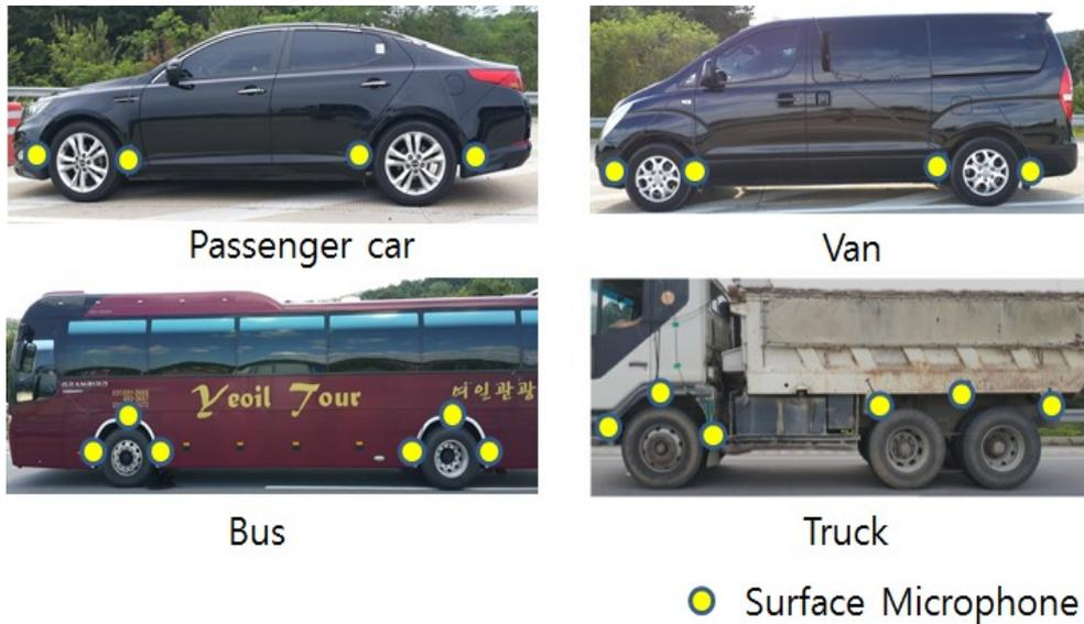
Figure 3 - Surface Microphone Position by Car Type
