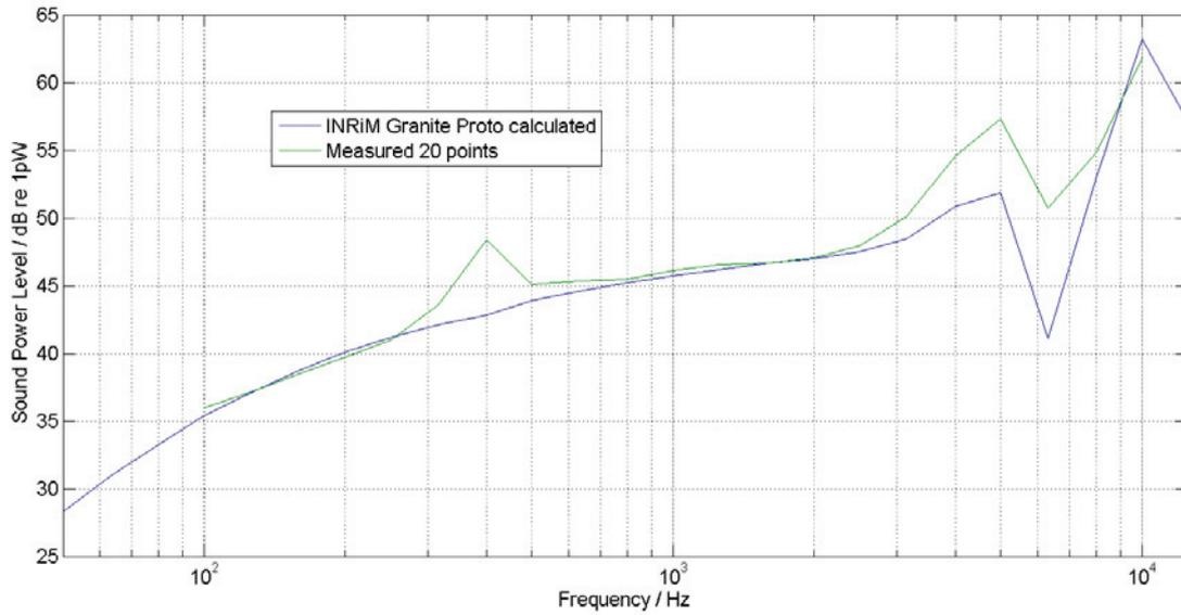
Fig.2.2 - Measured (green curve) and calculated sound power of an INRiM prototype of primary source
