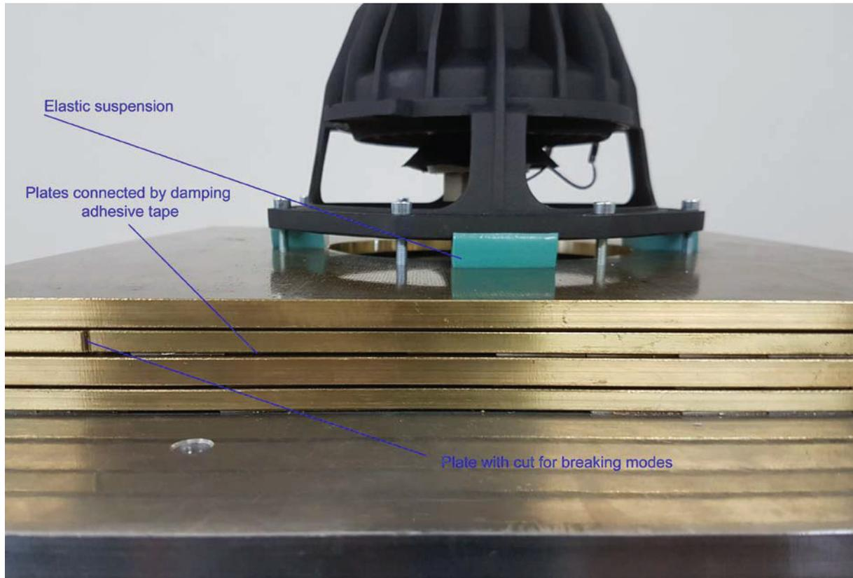
Fig. 2.3 - Example of multi layer mounting plate realization
