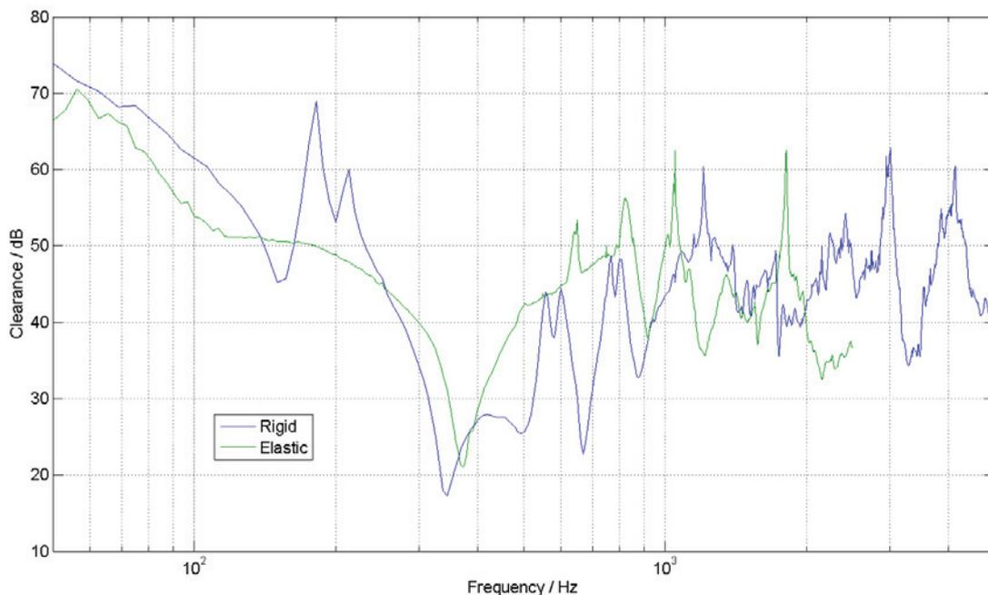
Fig.2.1 - Difference between piston velocity and velocity of the surrounding surface of an INRiM prototype of primary source
