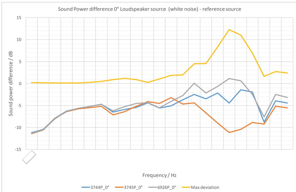
Fig. 5.1 - Difference of sound power between a reference sound source and a broadband directive source measured according to 3 ISO standards
