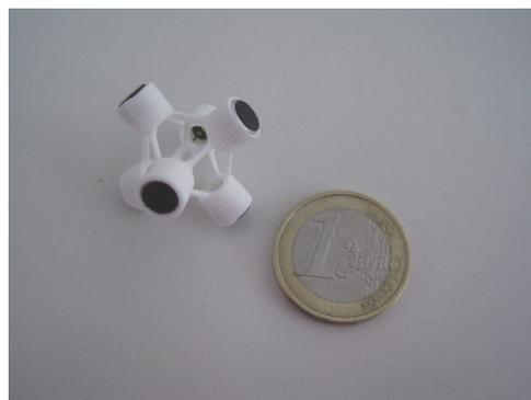
Figure 4. Three-dimensional low-cost pp-probe
