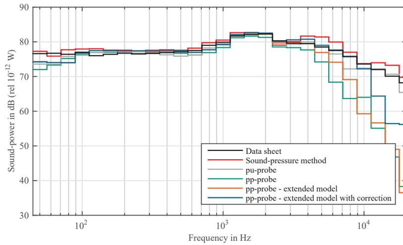
Figure 8. Evaluation of the measured sound-power of the reference source in terces
