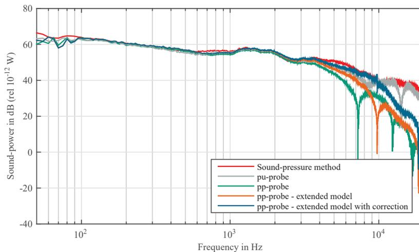
Figure 9. Narrow band evaluation of the measured sound-power of the reference source
