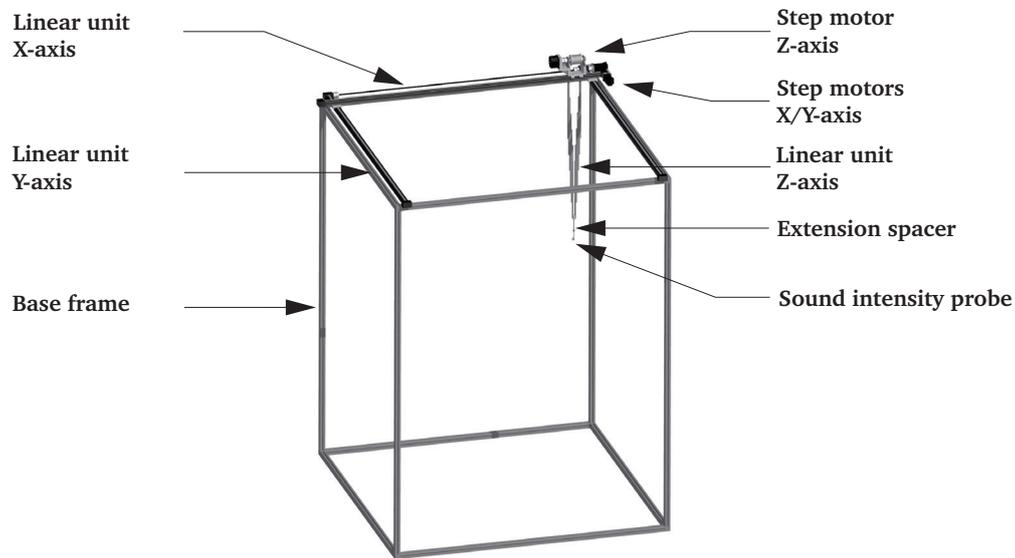
Figure 7. Portal system of the sound-intensity scanner
