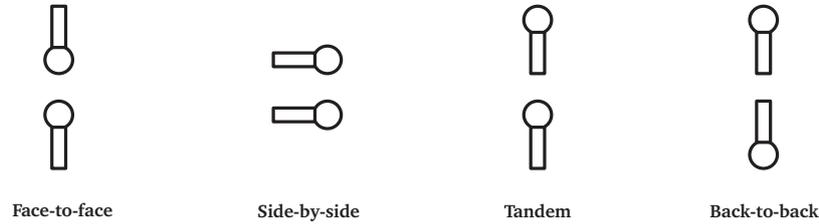
Figure 2. Schematic microphone orientation of pp-intensity probes
