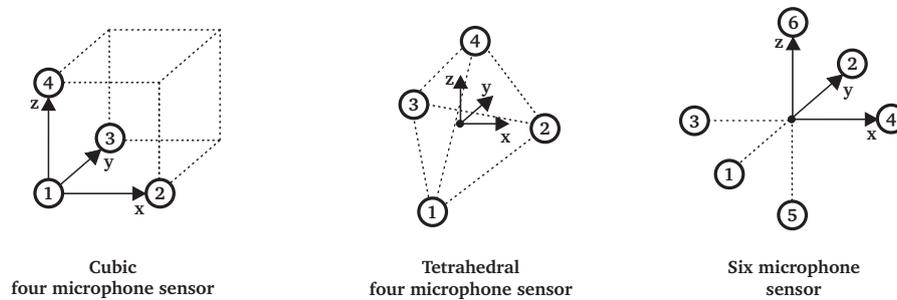
Figure 3. Schematic microphone orientation of 3D-pp-intensity probes
