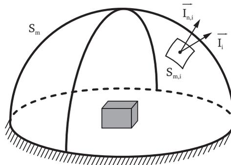
Figure 1. Enveloping surface for sound-power measurement based on the sound-intensity
