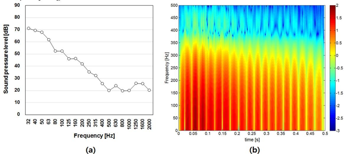
Figure 3 – Frequency response of impact noise generated by impact ball at S1
