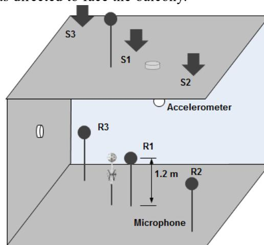
Figure 2 – Source and receiver positions for measurements
