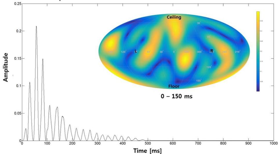
Figure 4 – Response of the noise generated by an impact ball and acoustic visualization result
