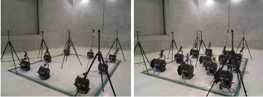
Figure 1 – 1 kW and 2 kW lighting equipment in the reverberation chamber.
