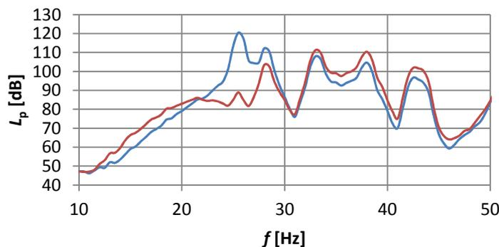
Figure 6 – Frequency response of the reverberation chamber; blue = without equalization, red = with equalization
