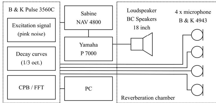
Figure 3 – Block diagram of measuring chain
