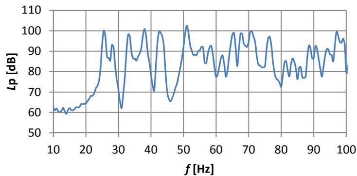
Figure 1 – Measured frequency response of the reverberation chamber
