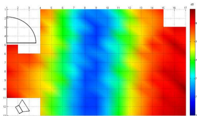
Figure 2 – Axial mode with frequency 25.5 Hz
