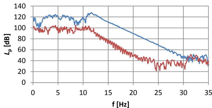
Figure 5 – Decay curves; blue = without equalization, red = with equalization
