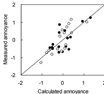
Figure 3 - Relationship between measured and calculated annoyance using linear combination of ACF and IACF factors. ●: Ball; ○: Bang.
