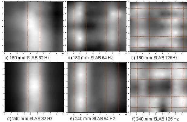
Figure 2 - Distribution contour of impact SPL driven by the center position
