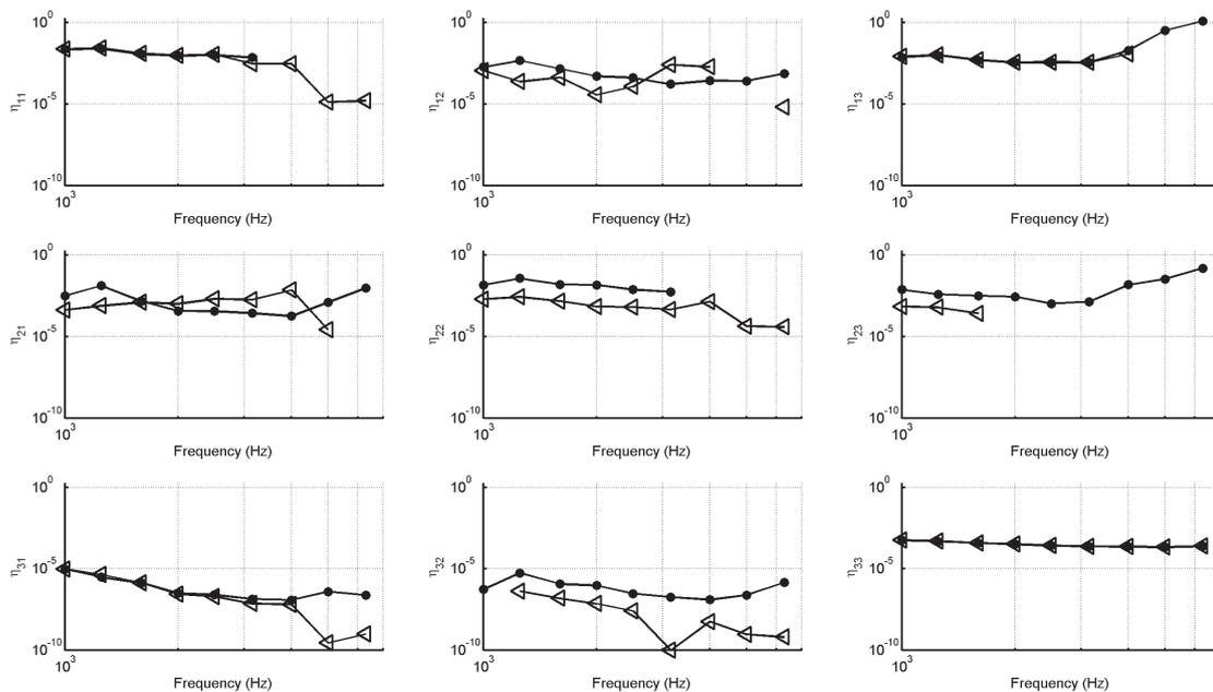
Figure 5 – SEA loss factors determined by the error minimisation method,  $J_J$ , ( $- \triangle -$ ) compared to the values obtained with PIM ( $- \bullet -$ ) (negative values not displayed)
