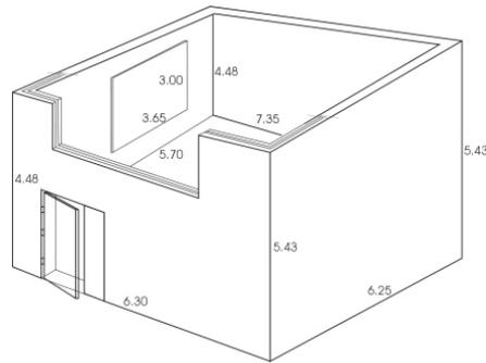
Figure 2 – Dimensions (metres) of ITEFI/CSIC Reverberant chamber
