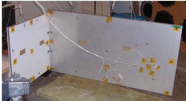
Figure 1 – L-shaped structure made up of two sandwich panels joined by two points
