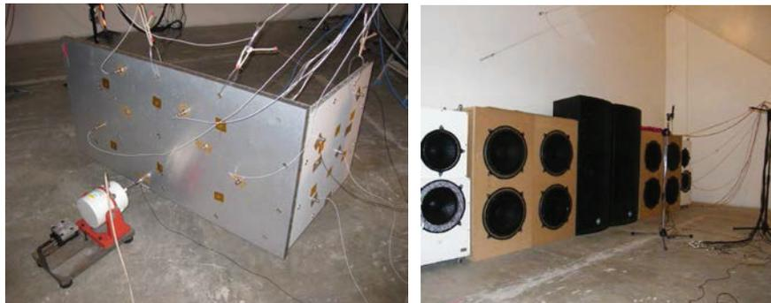
Figure 3 – Structural and acoustic excitation for the PIM test
