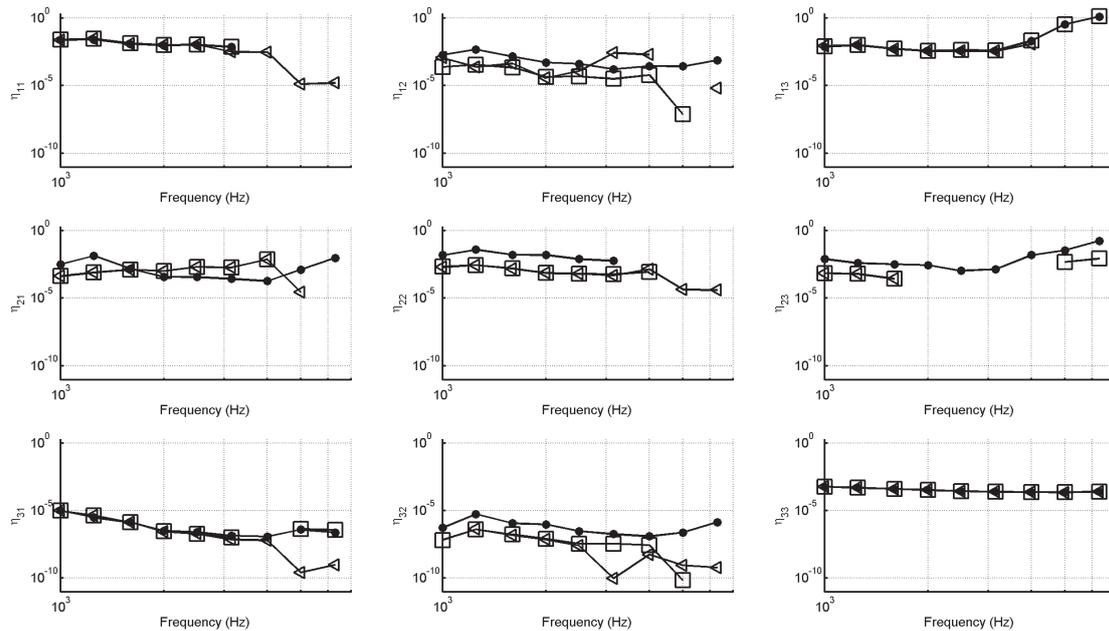
Figure 6 – SEA loss factors determined by updating law ( $\square$ ),  $J_2$ ; values obtained minimising the error ( $\triangle$ ),  $J_1$  and the values obtained with PIM ( $\bullet$ ) (negative values not displayed)
