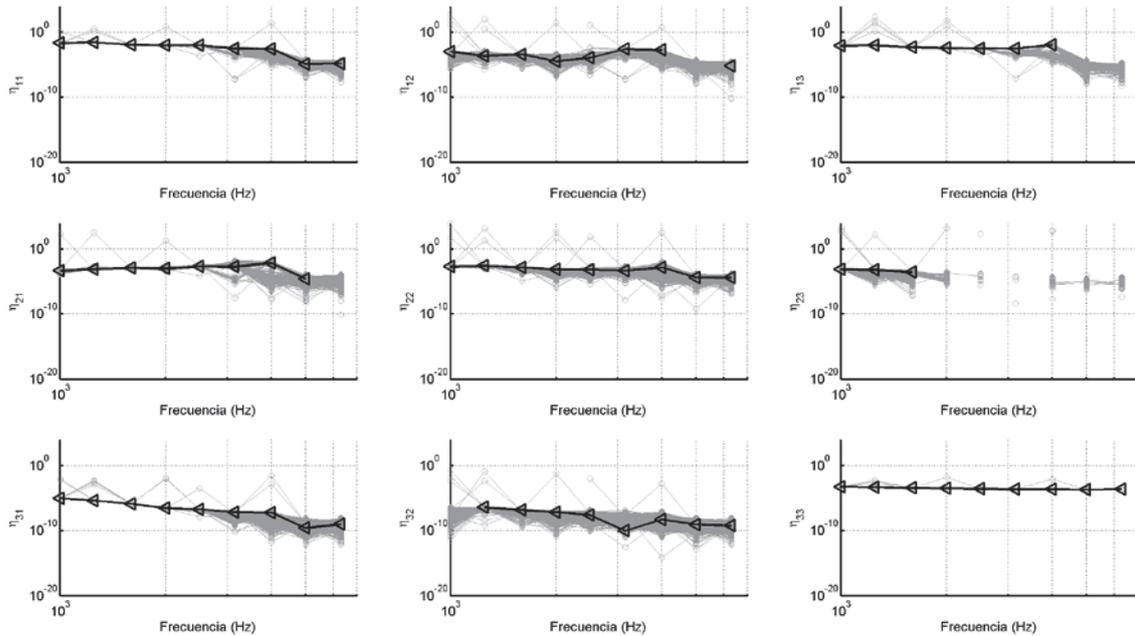
Figure 7 – SEA loss factors determined minimising the error in the power balance equation ( $J_1$ ) from the nominal energy (-◄-) and the Monte Carlo sample (-○-) (negative values not displayed)
