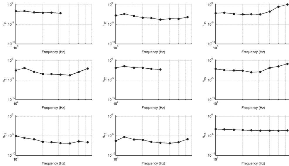
Figure 4 – SEA loss factors determined by means of PIM for successive input power in each subsystem (negative values not displayed)
