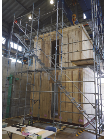
Figure 1 – Outside View of the cross laminated timber model building
