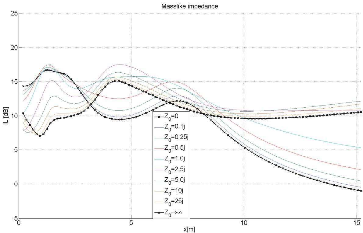
Figure 6 – IL of a barrier on a mass-like ground
