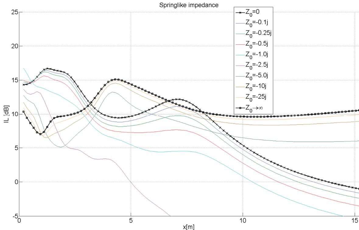
Figure 7 – IL of a barrier on a spring-like ground
