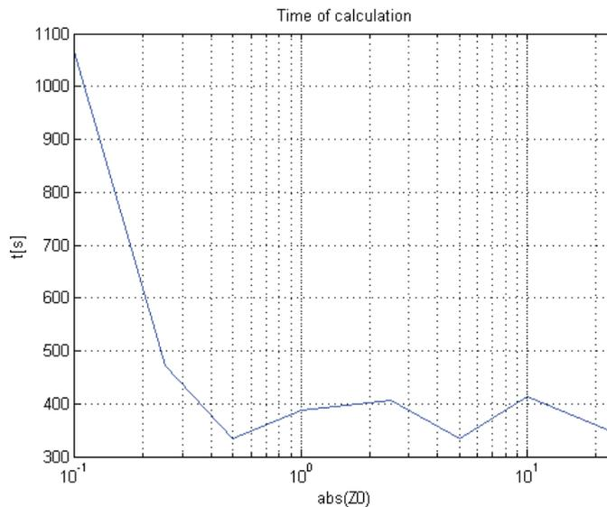
Figure 4 – Calculation time for different values of  $|Z_0|$  of the spring-like impedance
