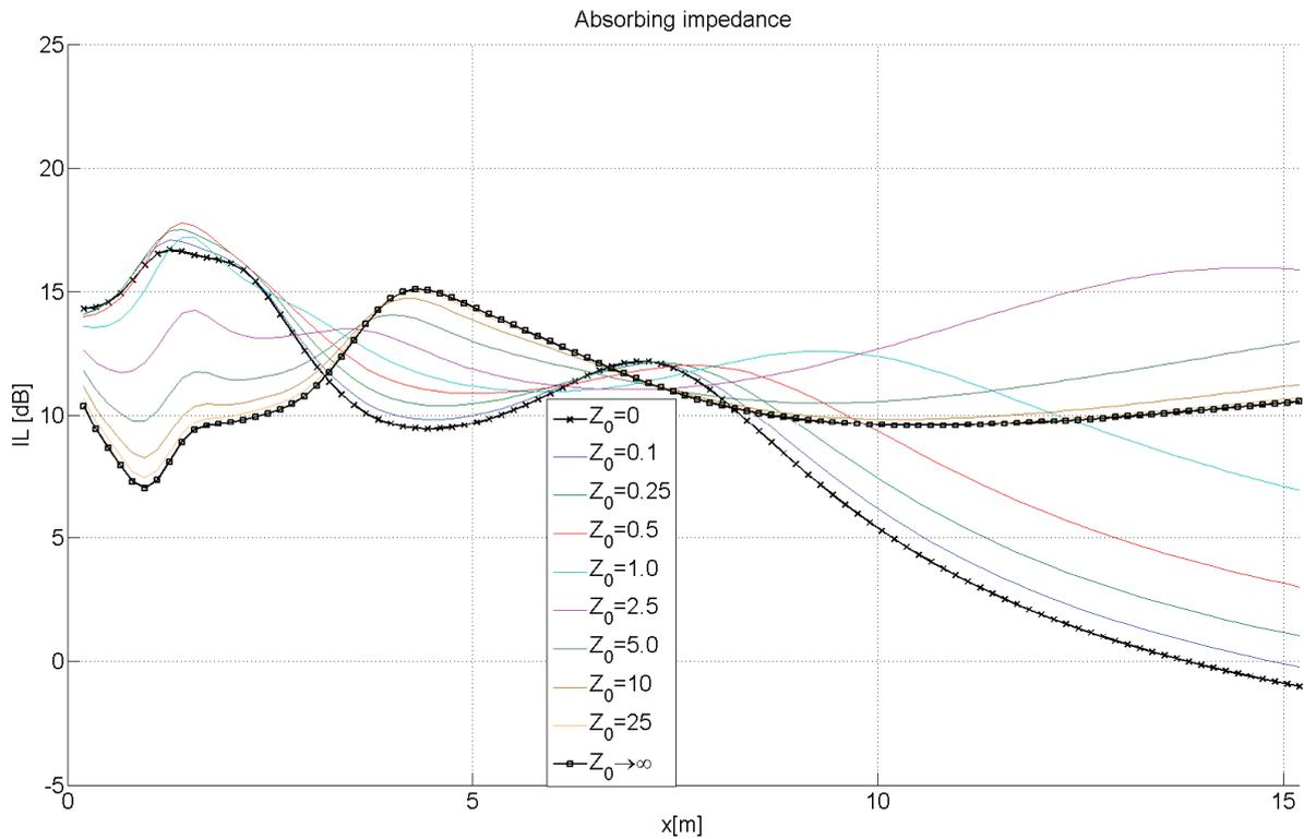
Figure 5 – IL of a barrier on absorbing ground
