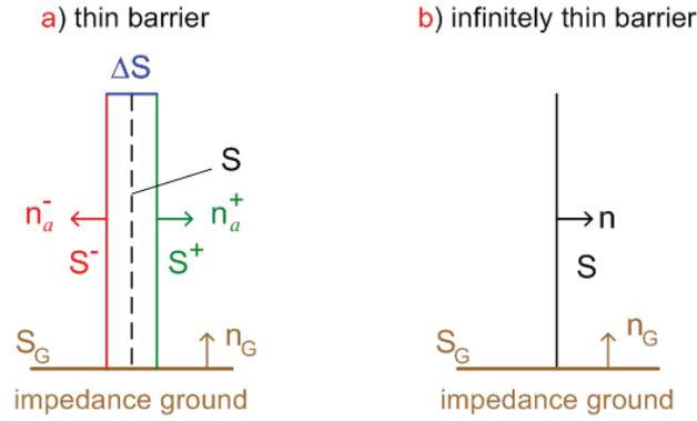
Figure 1 – Model of the sound barrier
