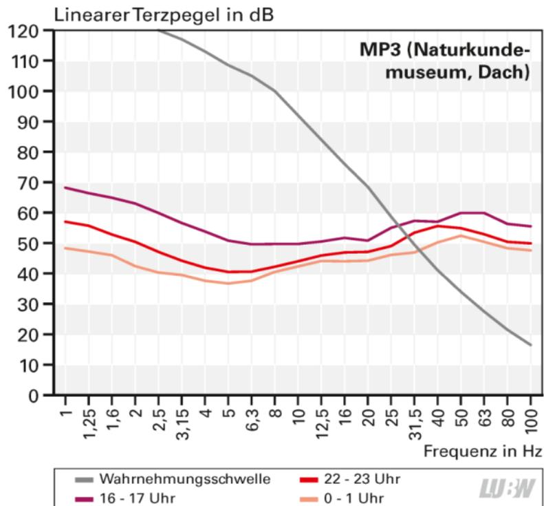
Figure 8: Linear third-octave band spectrum inner city of Karlsruhe, measured on a roof at different times. Perception threshold (grey).
