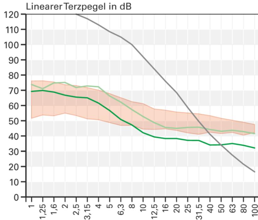
Figure 9: Comparison of the noise situation in the free field (green – without WT in the vicinity) with the level range of a WT at a distance of 300 m (red). Perception threshold (grey).
