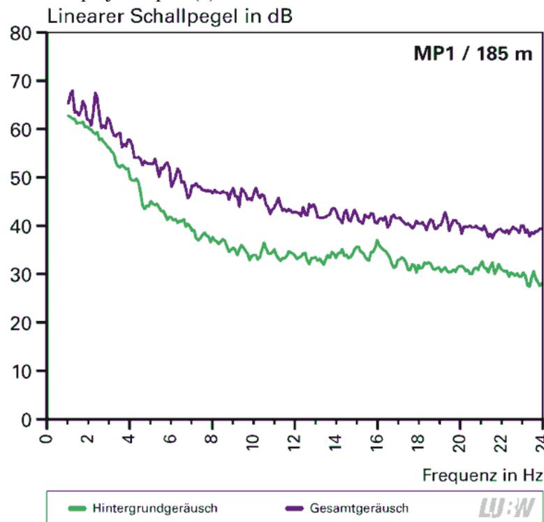
Figure 1 - Narrow-band spectrum (resolution 0.1 Hz). Total noise (violet, upper curve) with WT in operation and background noise (green, lower curve) with WT out of operation, measured in near sound field at a distance of 185 m to the turbine. The discrete frequencies below 6 Hz are easily visible (upper curve).
