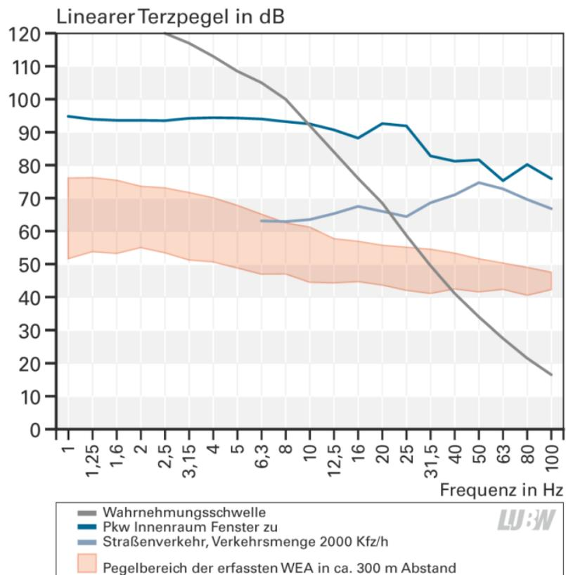
Figure 6: Third-octave band spectrum road traffic at the permanent measuring station Reutlingen (blue curve center) with 2,000 vehicles/h. Results of the WT measurements (red) and level inside a running passenger car with closed windows (upper blue curve). Perception threshold (grey).
