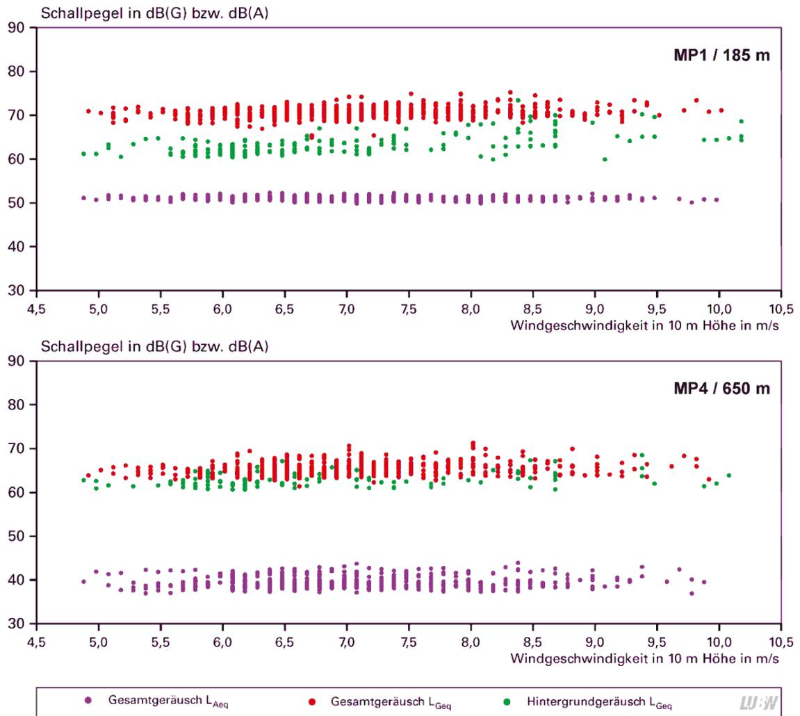
Figure 3 - A-level (violet dots) and G-level (red dots with WT in operation, green dots with WT out of operation). At a distance of 185 m (upper diagram), significant differences in the G-level between WT in and out of operation can be seen. At a distance of 650 m, there are only minor differences (lower diagram).
