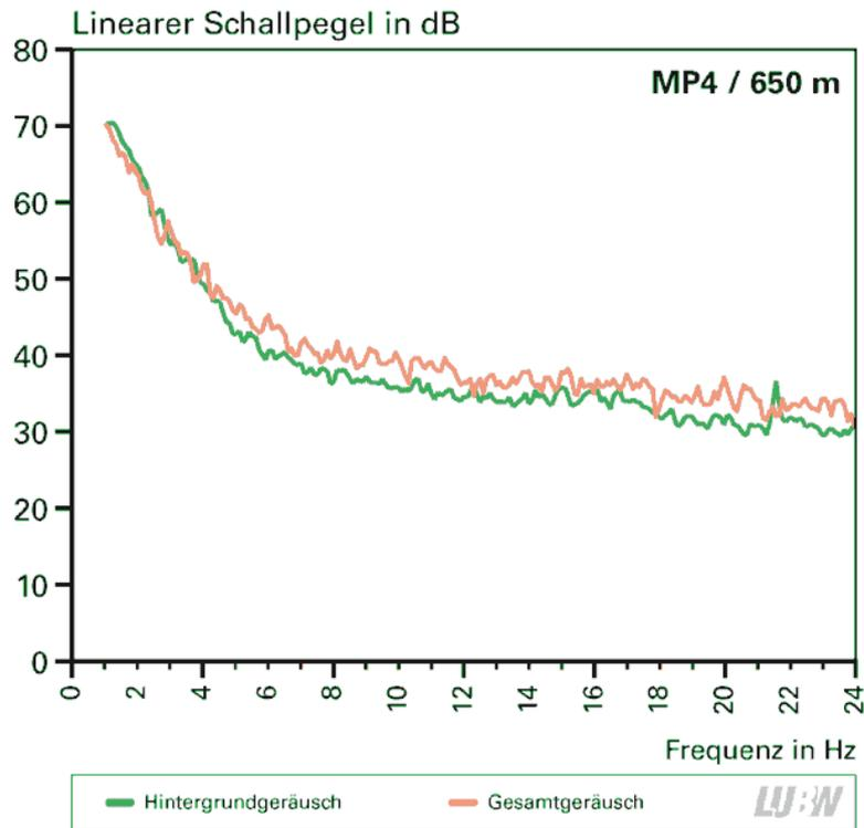
Figure 2 - 0.1-Hz narrow-band spectrum of total noise (orange, upper curve – with WT in operation) and background noise (green, lower curve – with WT out of operation) measured at a distance of 650 m.
