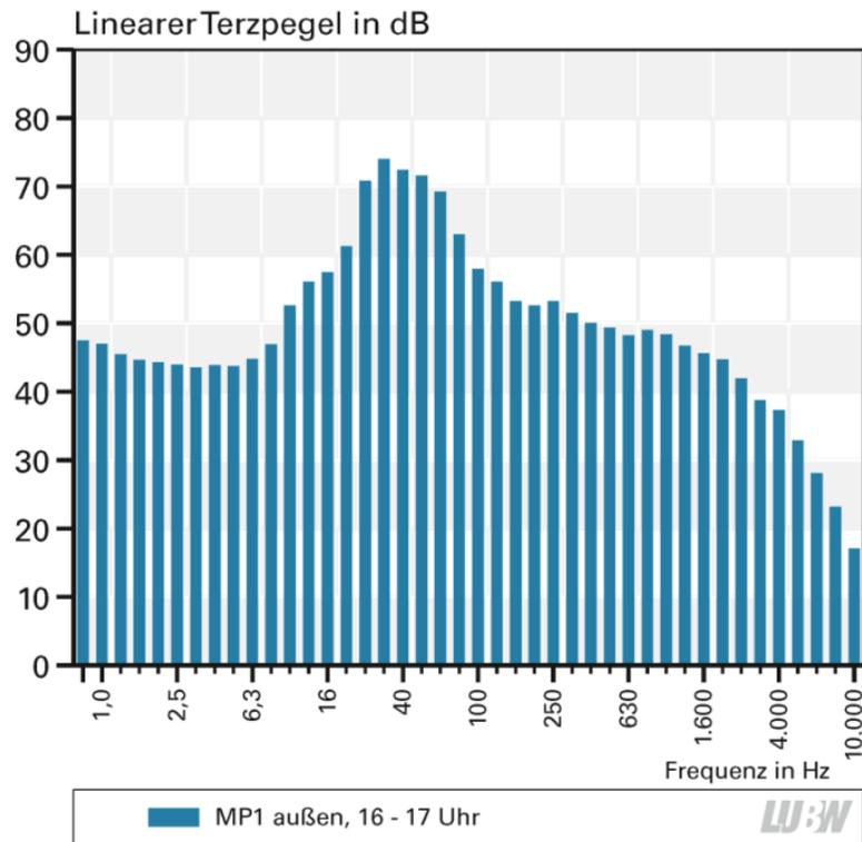
Figure 5: Third-octave band spectrum road traffic (immission), recorded on weekdays between 16:00 and 17:00. The traffic intensity is 14,000 vehicles/24h with a percentage of trucks of 3 %.
