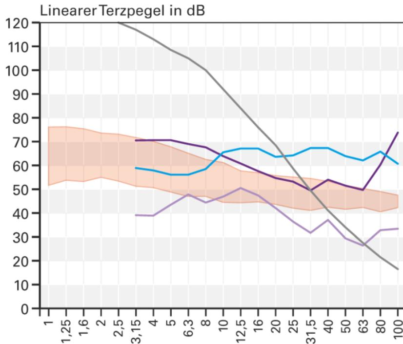
Figure 10: Third-octave band spectra of oil-fired heating (violet), washing machine (blue) and gas-fired heating (lowest curve). For comparison WT (red), perception threshold (grey).
