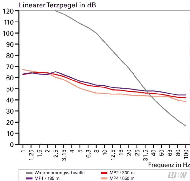
Figure 4: Third-octave band spectra of the total noise measured at distances of 185 m, 300 m and 650 m to the WT. For comparison purposes, the perception threshold was additionally included in the figure (grey).
