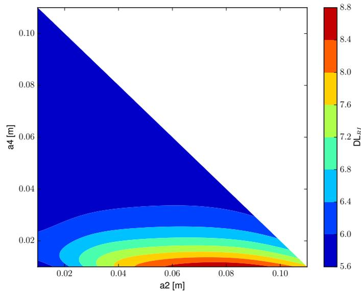
Figure 4 – Subset of the  $DL_{RI}$  data for constant absorber parameters ( $a_1 = a_5 = 0$  and  $a_2 + a_4 \leq 11$  cm)
