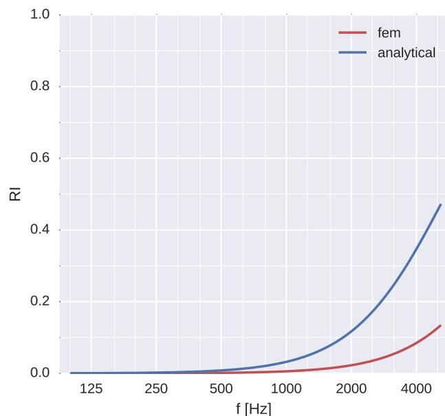
Figure 2 – Comparison of the reflection index of a perforated plate with a hole ratio of 30 %
